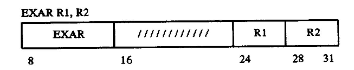
The millicode access register specified by R1 is loaded from the program access register specified by R2.
