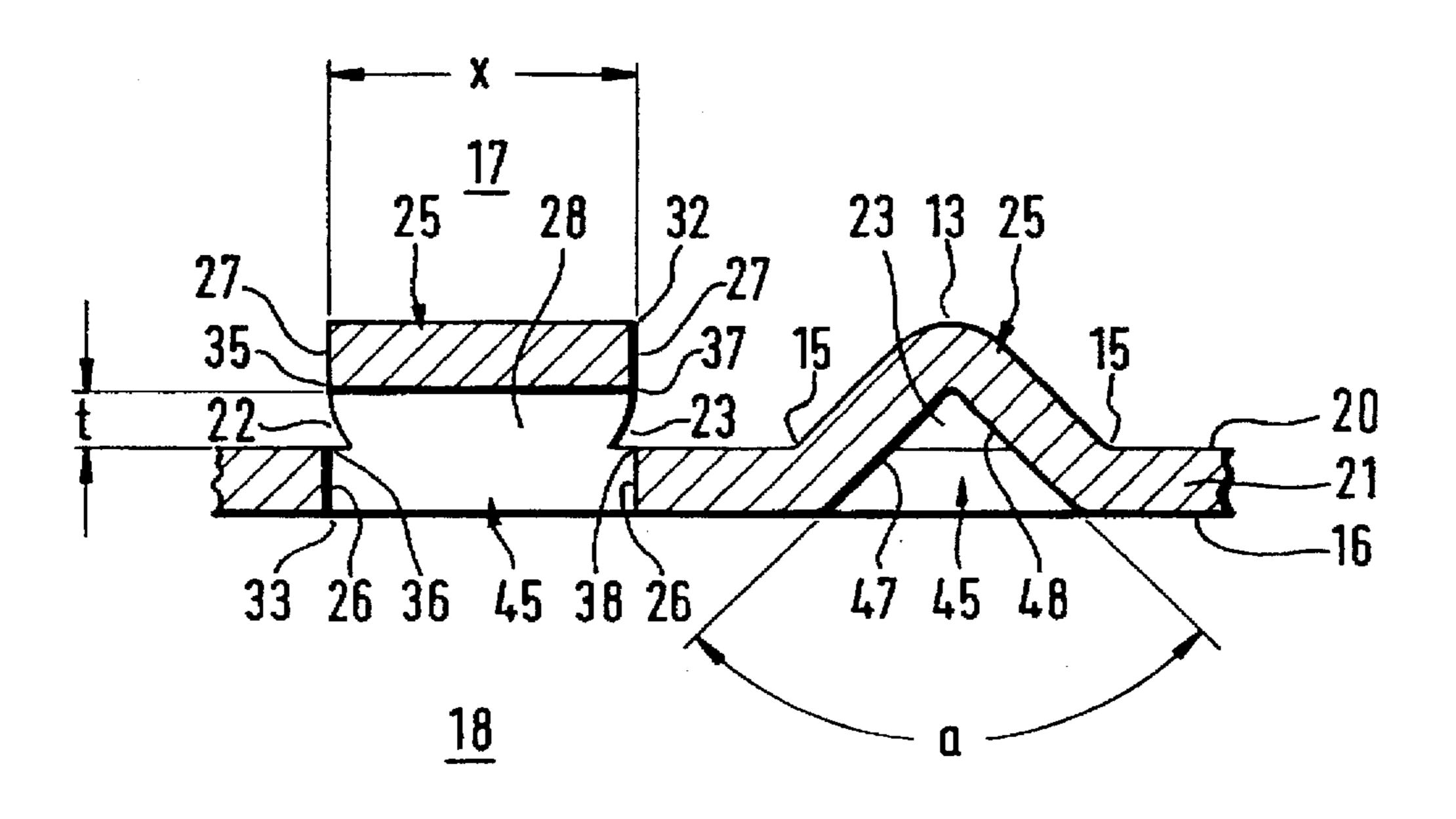
The filtering means of the present invention affords ease and economy of manufacture, requiring only a single operation to produce on a filtering means a plurality of apertures with a plurality of domes.
