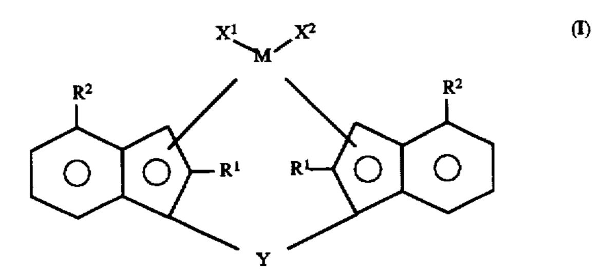
wherein M is a transition metal; R1 is a hydrocarbon group of 2 to 6 carbon atoms, R<sup>2</sup> is an aryl group of 6 to 16 carbon atoms; X1 and X2 are each a halogen atom or the like; and Y is a divalent hydrocarbon group, a divalent siliconcontaining group or the like.
