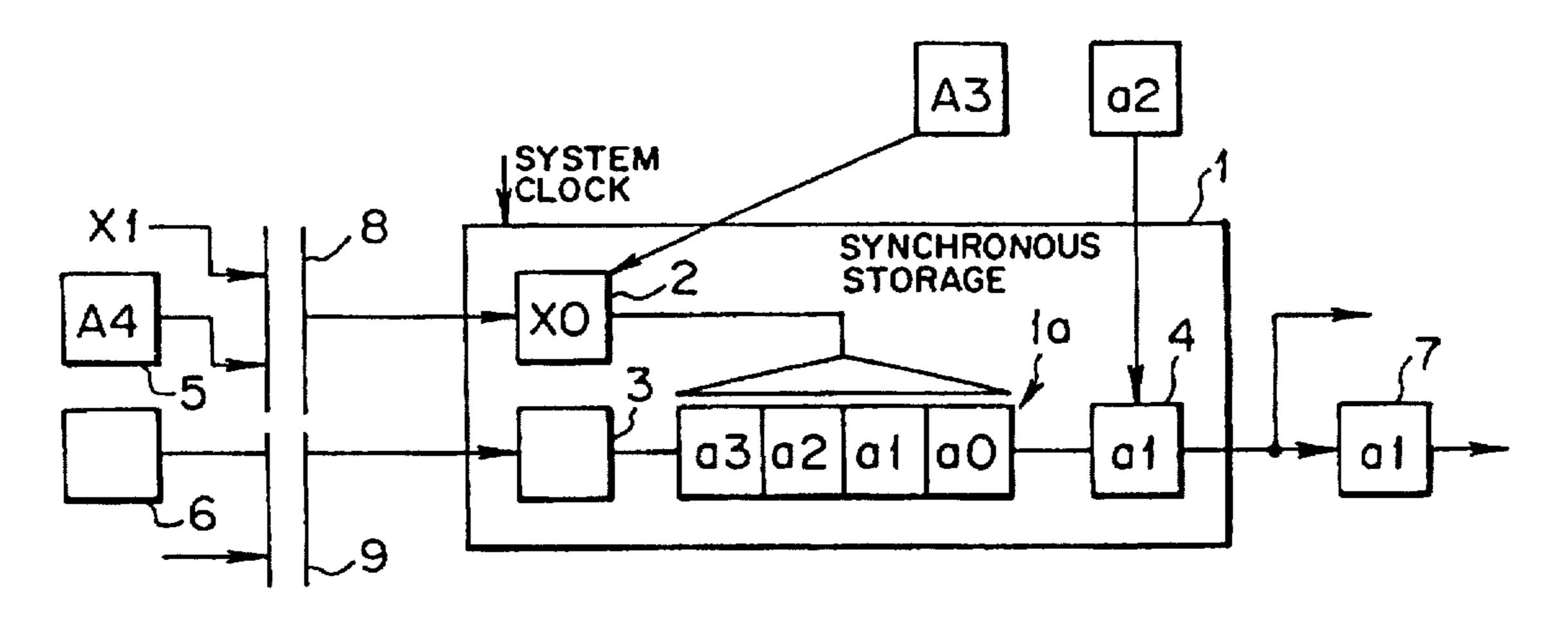
INFORMATION PROCESSING APPARATUS INCLUDING SYNCHRONOUS STORAGE HAVING BACKUP REGISTERS FOR STORING THE LATEST SETS OF INFORMATION TO ENABLE STATE RESTORATION AFTER INTERRUPTION
