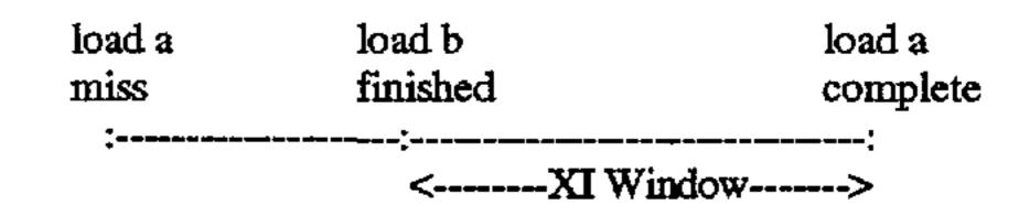
In the preferred embodiment, the "XI window" extends from the time when a load or store instruction causes a miss to the time when that load or store completes. This is shown graphically below:
