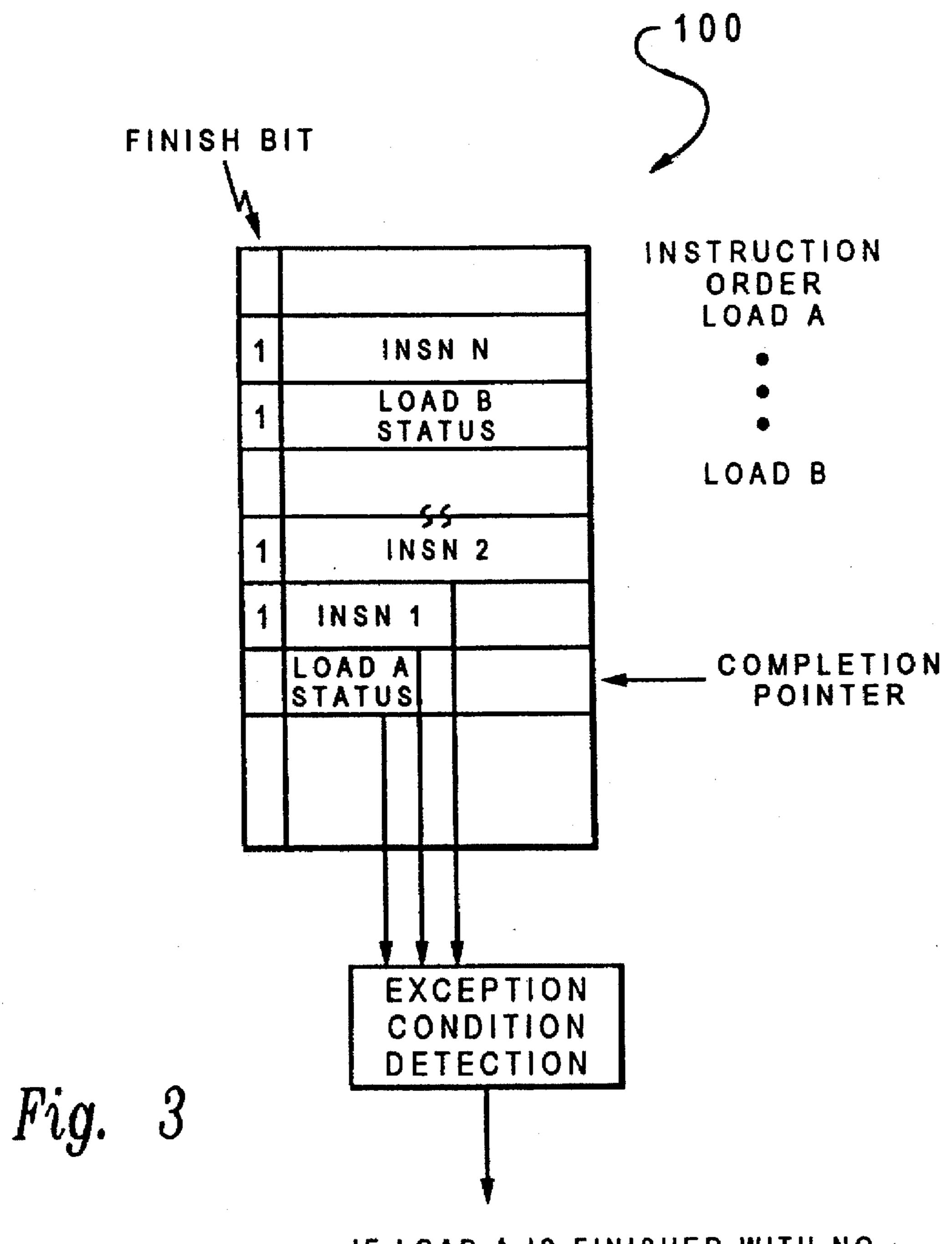
IF LOAD A IS FINISHED WITH NO X1 EXCEPTION THEN COMPLETE LOAD A AND SUBSEQUENT INSTRUCTION (INSN 1, INSN 2 ... LOAD B) ELSE RE-ISSUE LOAD A AND CANCEL ALL SUBSEQUENT INSTRUCTIONS
