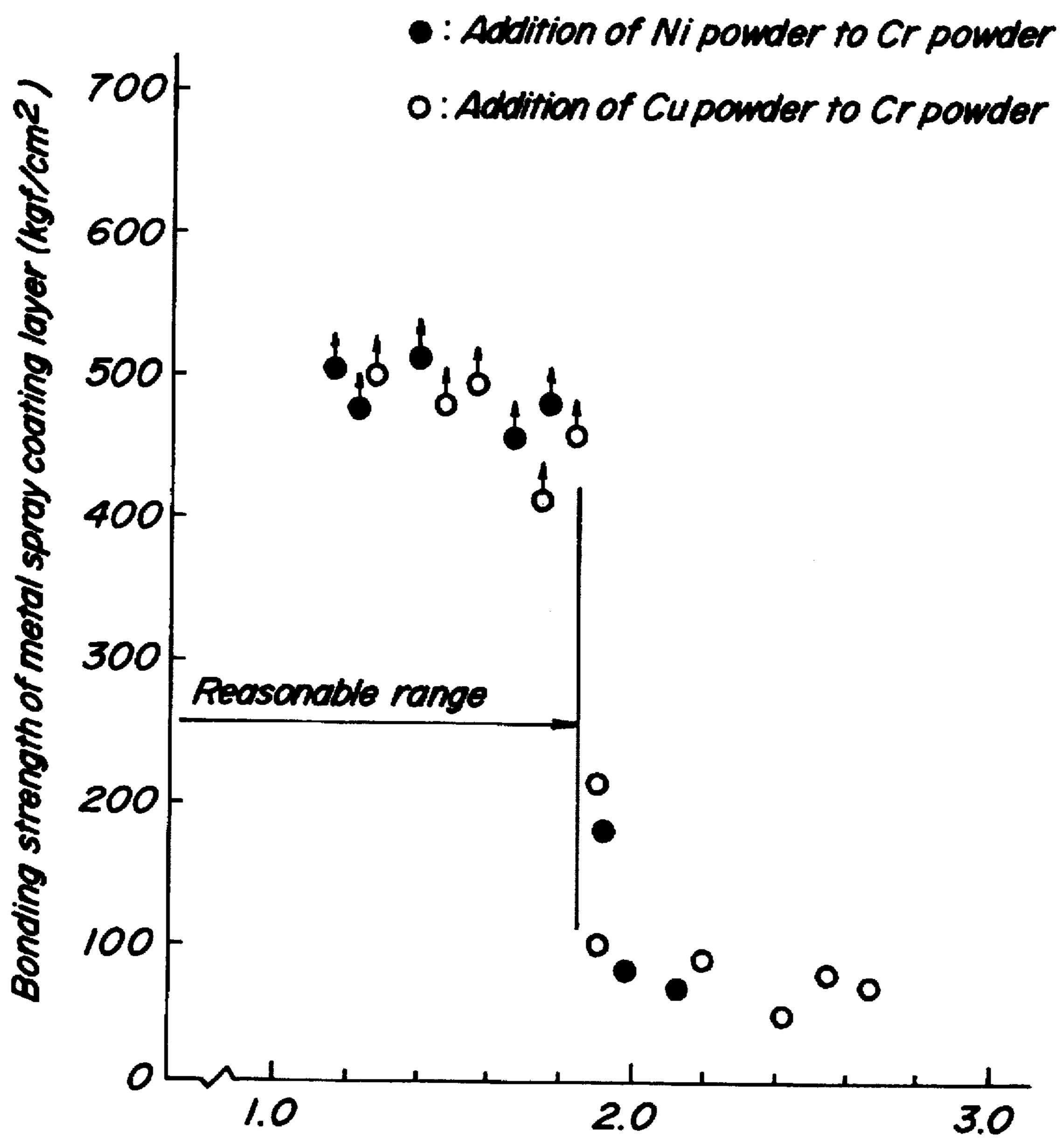
Linear expansion coefficient ratio of metal spraying material to carbon substrate
