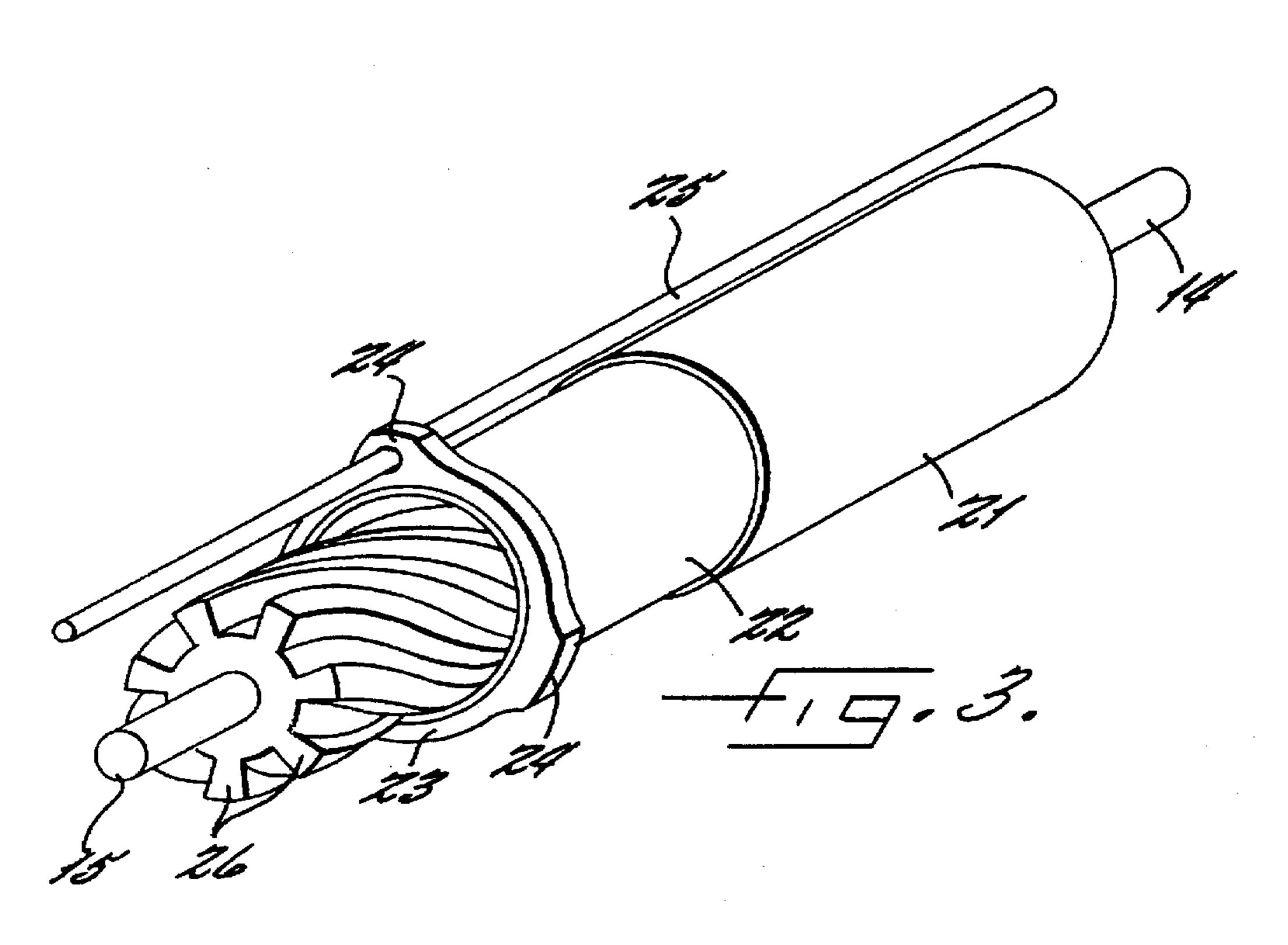
This invention relates to drive mechanisms and particularly to drive mechanisms adapted to provide a drive from one rotatable member to another at a speed difference.
