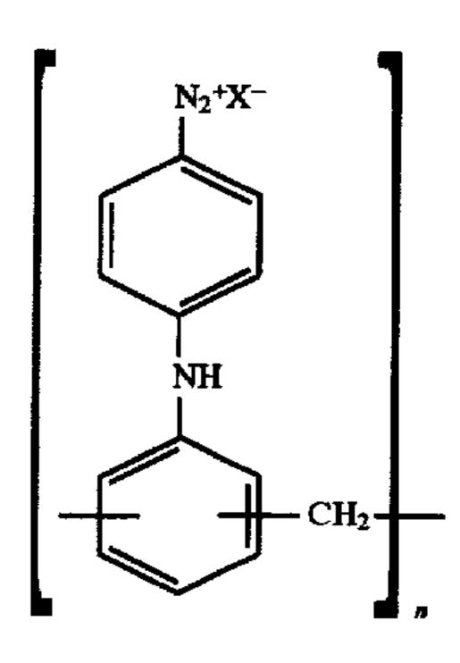
having a mixture or anions X<sup>-</sup> comprising from about 45 to about 94 mol percent ZnCl<sub>4</sub><sup>=</sup> and from about 6 to about 55 mol percent HSO<sub>4</sub><sup>-</sup>; and n ranges from about 2 to about 50 which comprises
