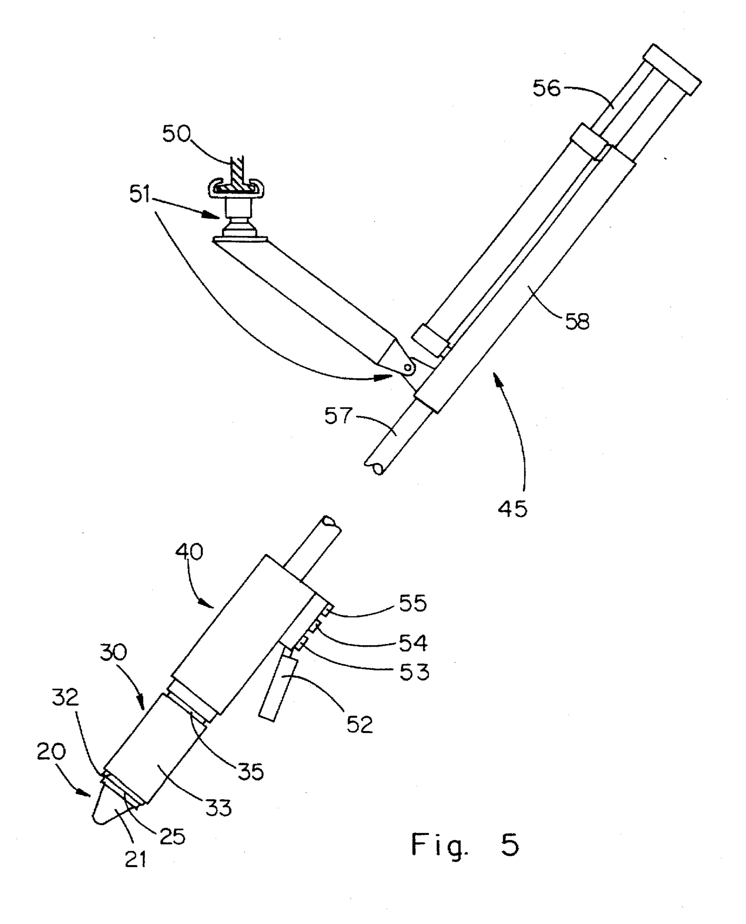
This invention relates to a process and apparatus for separating and dosing the rectum of a slaughtered animal carcass.
