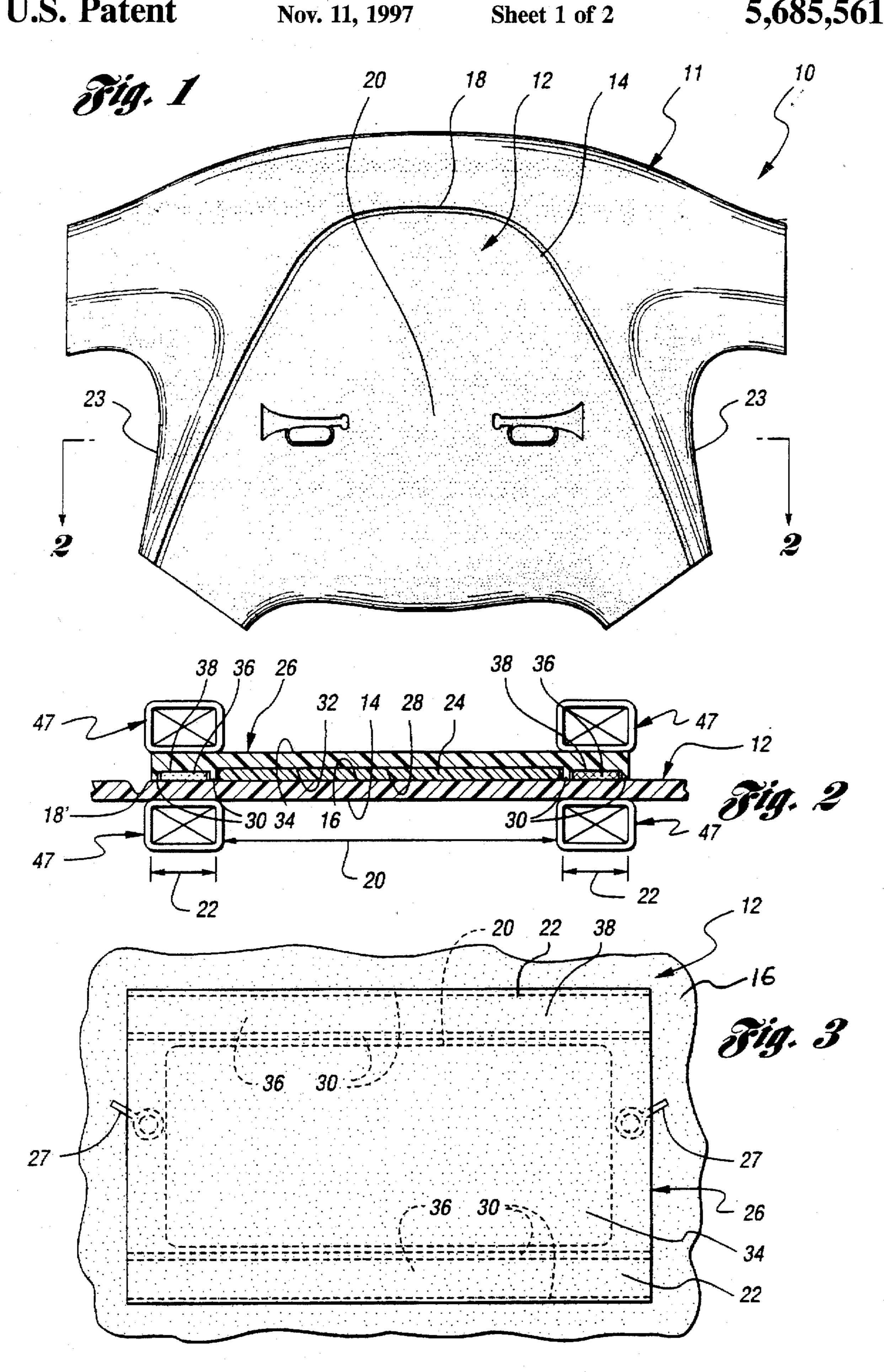
POSITION FRONT AND BACK PANELS SO INNER SURFACES OF PANELS ARE ADJACENT ONE ANOTHER
