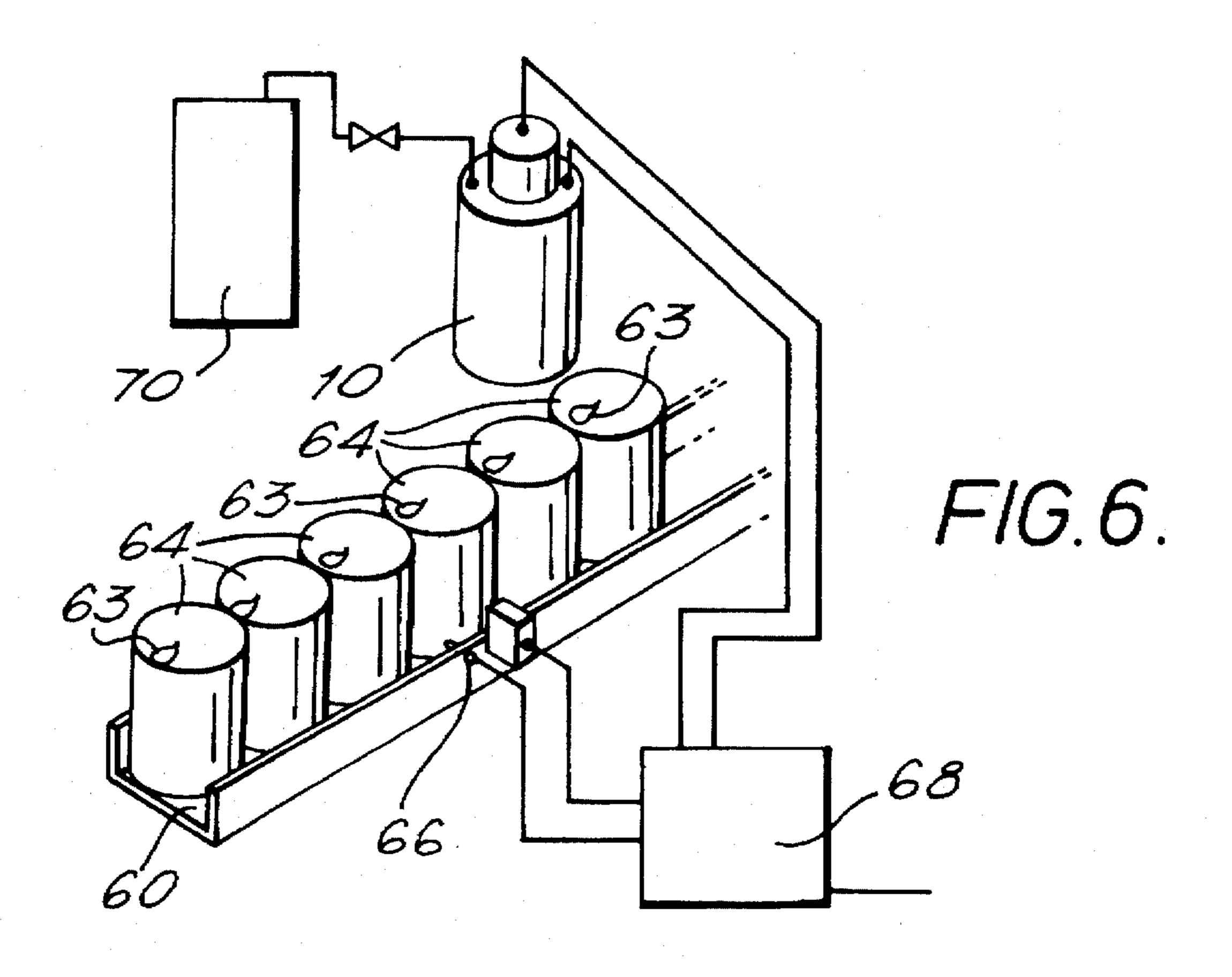
The present invention relates to apparatus for dispensing droplets of liquid and relates particularly, but not exclusively, to apparatus for dispensing droplets of chosen or suitable volume of a cryogenic liquid, for example, liquid nitrogen.
