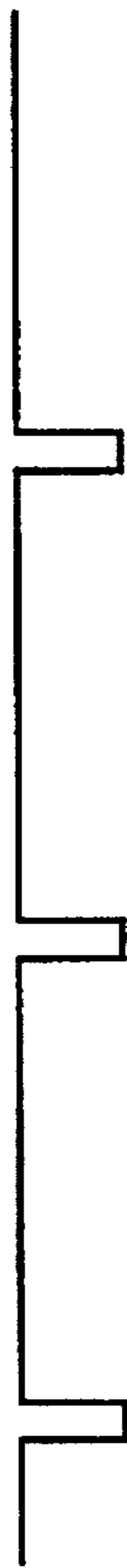
INVERTED VERSION OF SCANNING SIGNAL
