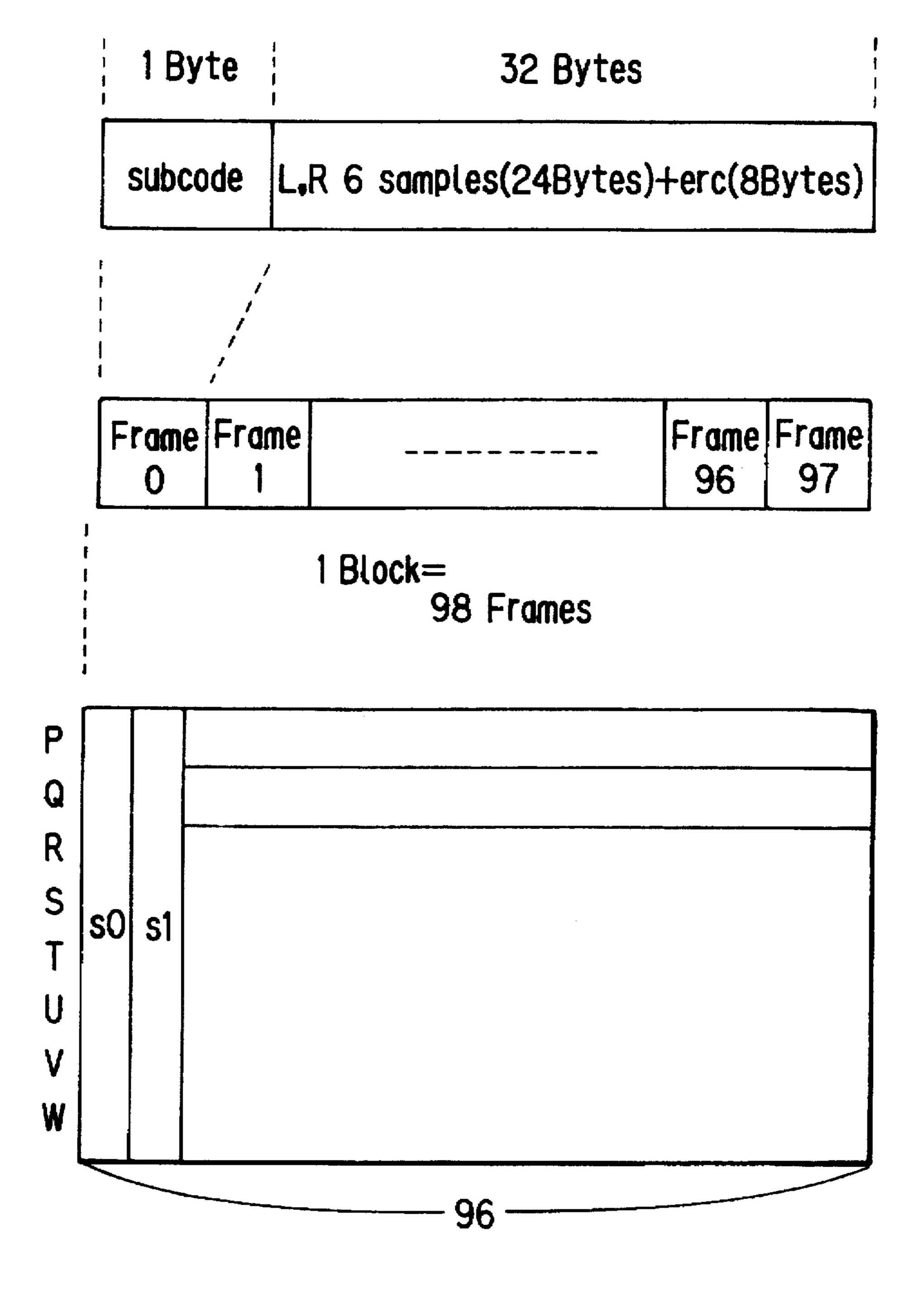
1 Block→75Hz 1 Frame→75×98Hz subcode bit rate=7.35 kBytes/s
