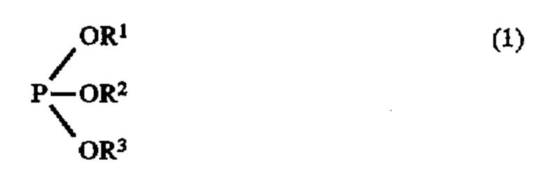
wherein R<sup>1</sup>, R<sup>2</sup> and R<sup>3</sup> independently of each other represent a substituted aryl group having at least 7 carbon atoms, the ratio of said rhodium compound (a) to said tris(substituted aryl) phosphite (b) ranging from 110 to 1000 moles per 1 gram atom of rhodium in said rhodium compound (a).
