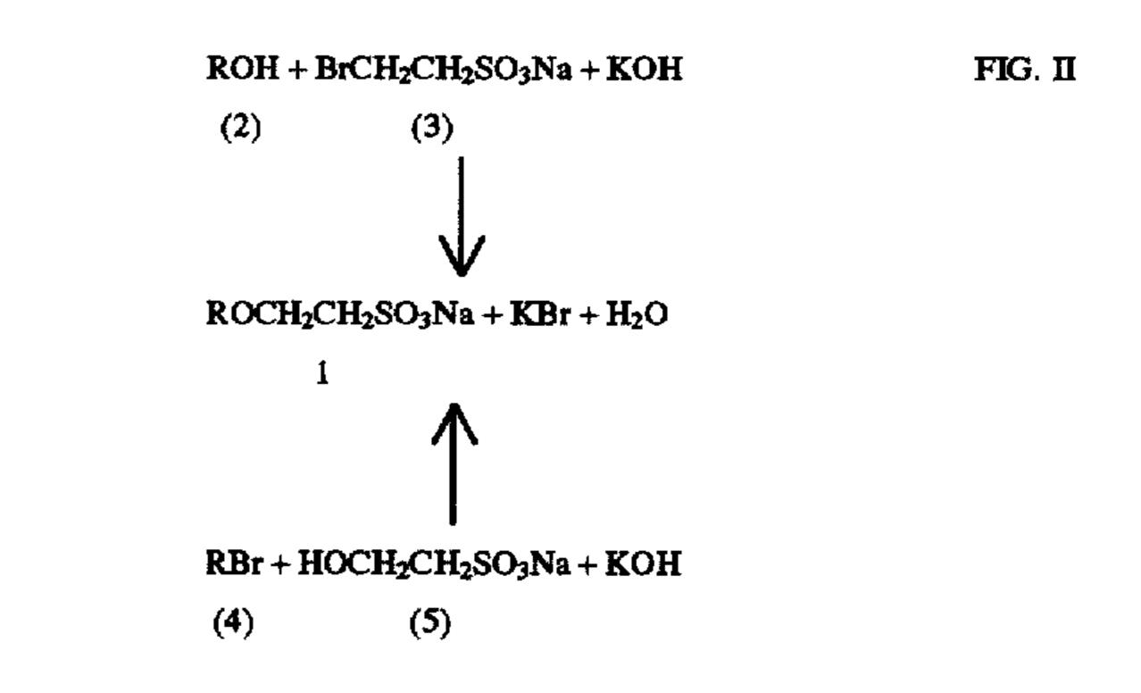
Suitable catalysts which can be employed include potassium hydroxide, tetrafluoroboric acid, mercury oxide, and bis-acetylacetonate nickel. Generally the reaction is preferably performed for an extended period of time. Temperatures of from about 25° C. to the reflux and stability termination temperature of the system can be employed. Preferably the temperature is about 50° C. to 90° C. The time of the reaction is dependent upon the catalyst, if present, and the temperature can be employed.
