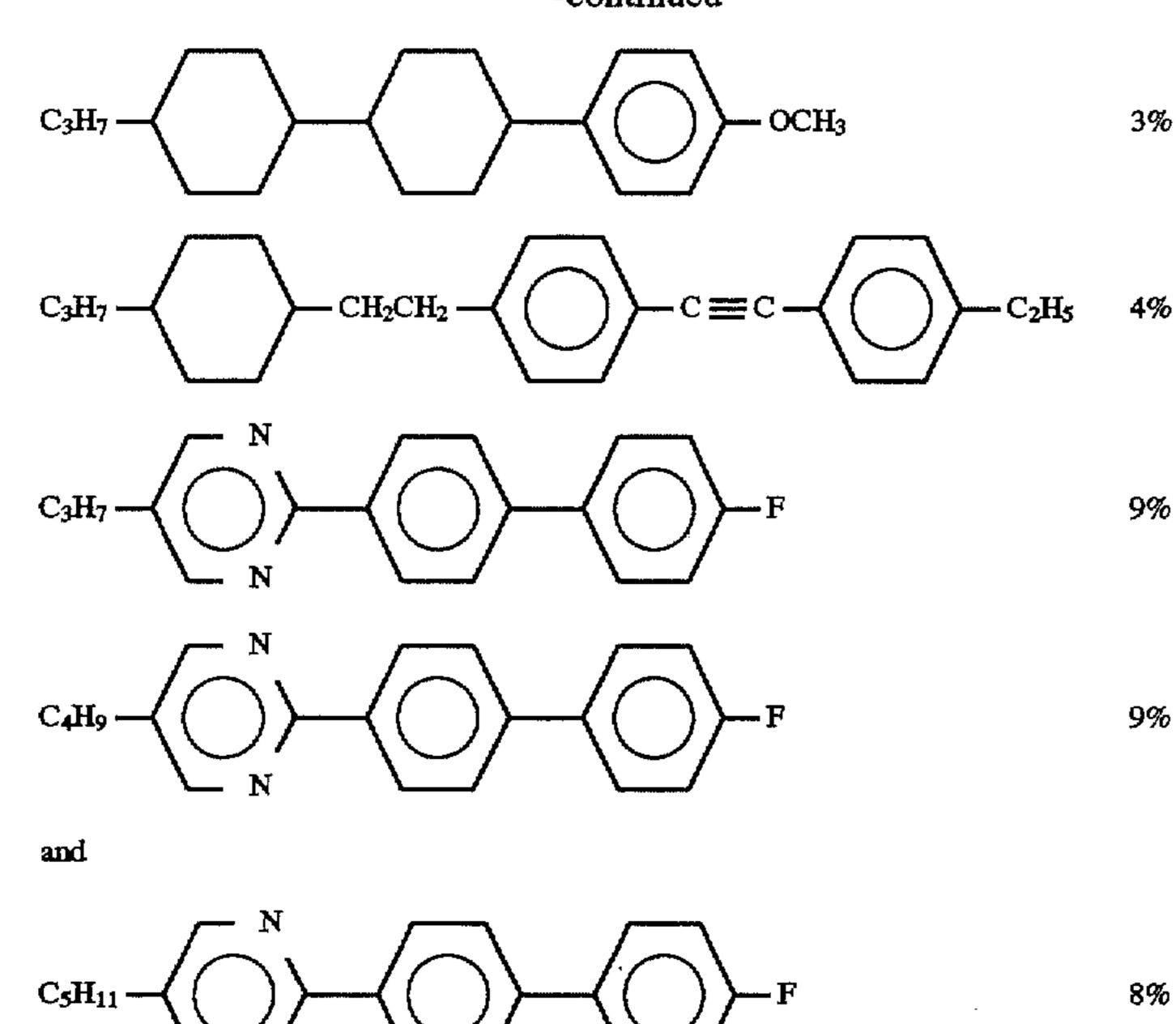
was prepared. A clearing point of the composition was 93.6° C. A viscosity, a dielectric anisotropy, and a threshold voltage each at 20° C., of the composition were 21.2 mPa.s, 9.2, and 1.90 V., respectively, and an optical anisotropy at 25° C. of the composition was 0.156.
