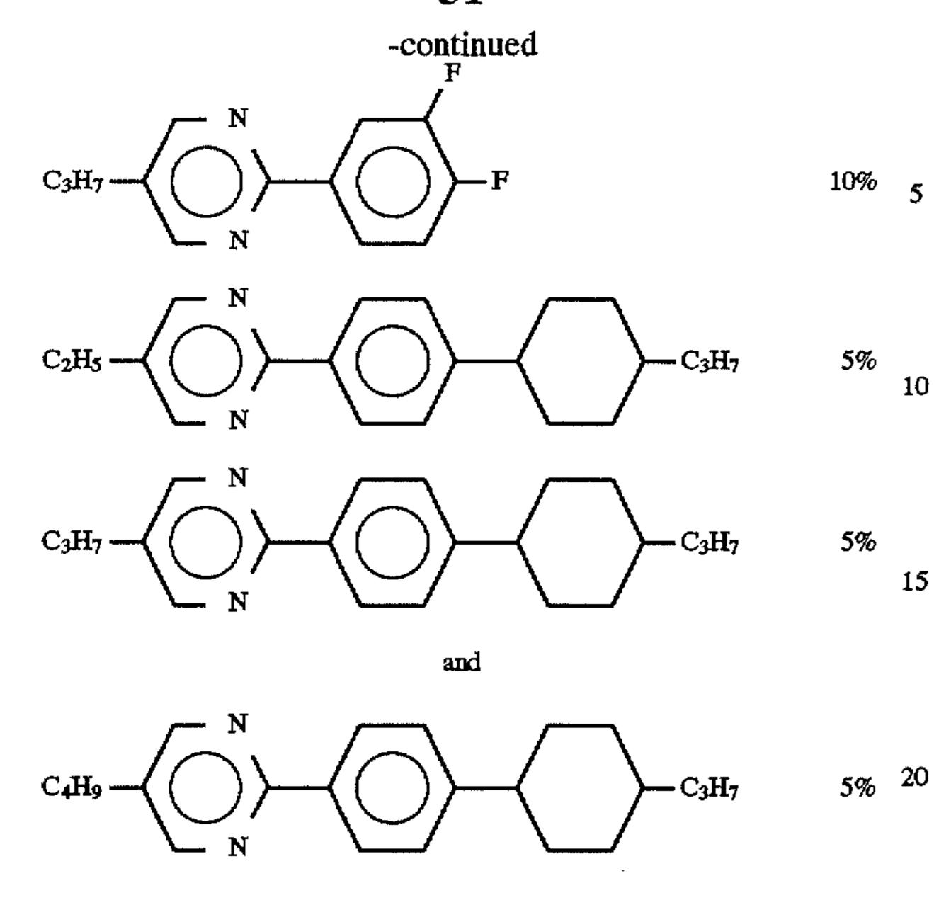
was prepared. A clearing point of the composition was 76.8° 25 C. A viscosity, a dielectric anisotropy, and a threshold voltage each at 20° C., of the composition were 17.3 mPa.s, 6.9, and 1.75 V., respectively, and an optical anisotropy at 25° C. of the composition was 0.133.
