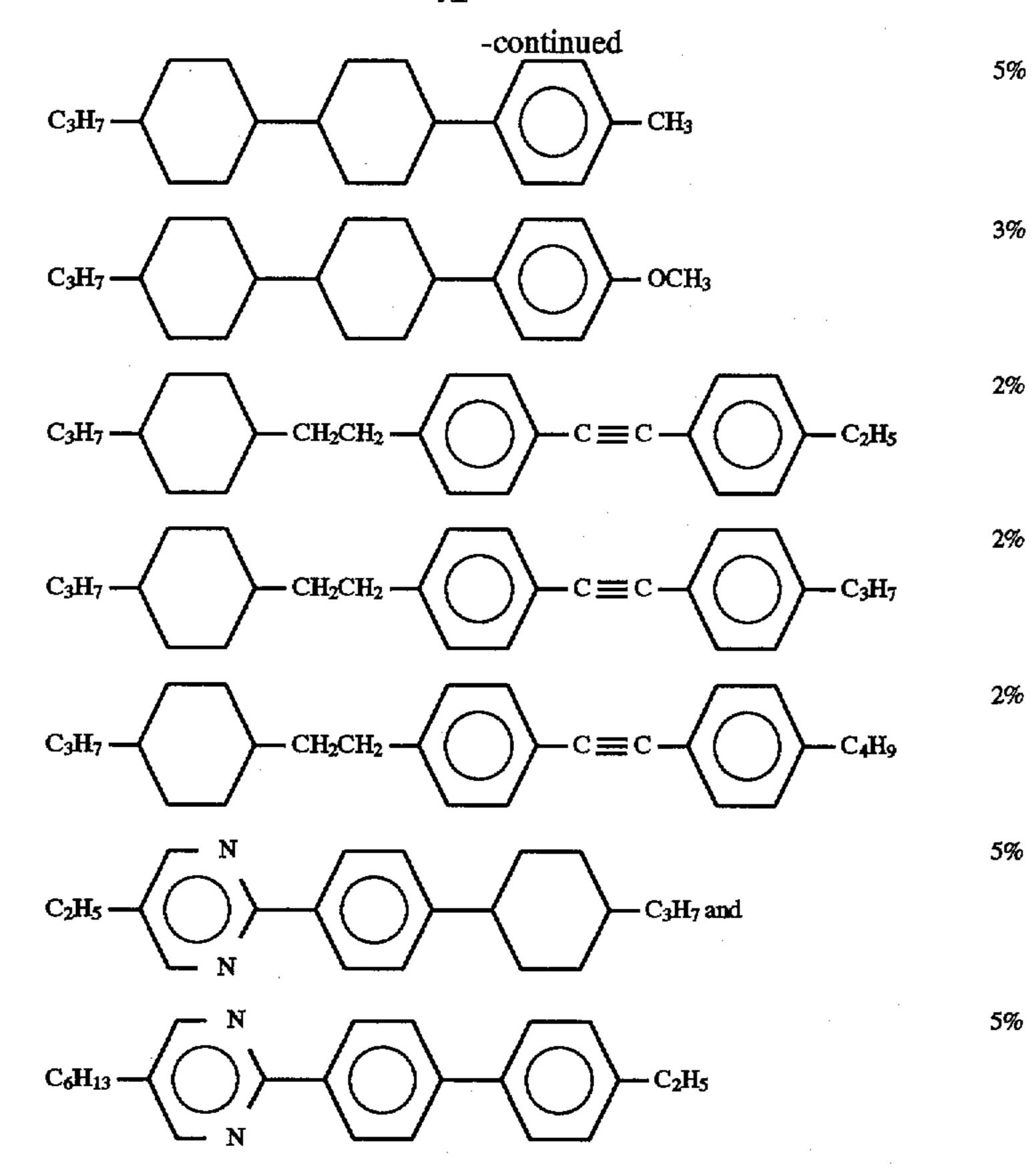
was prepared. A clearing point of the composition was 119.5° C. A viscosity, a dielectric anisotropy, and a threshold voltage each at 20° C., of the composition were 22.0 mPa.s, <sup>35</sup> 10.7, and 2.01 V., respectively, and an optical anisotropy at 25° C. of the composition was 0.144.
