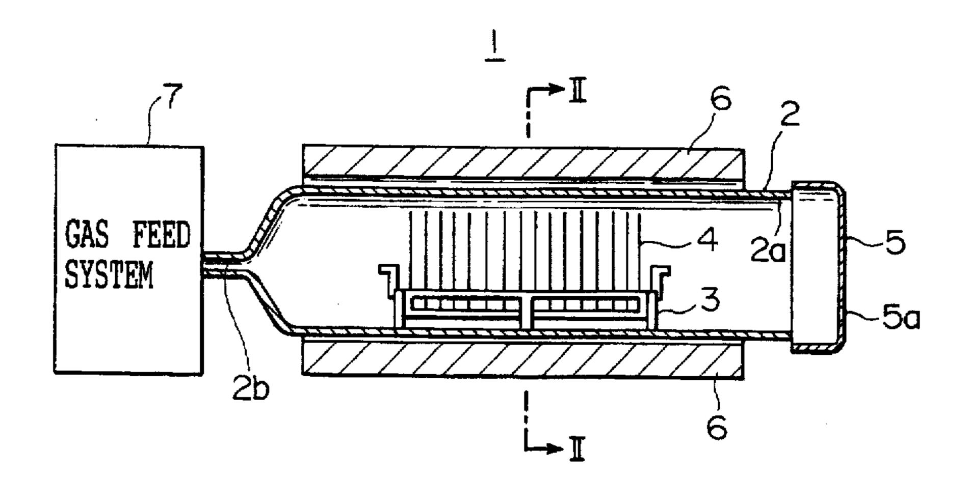
apparatus reduce and control the fixed-charge density in the oxide film of a MOS device with a high repeatability.
