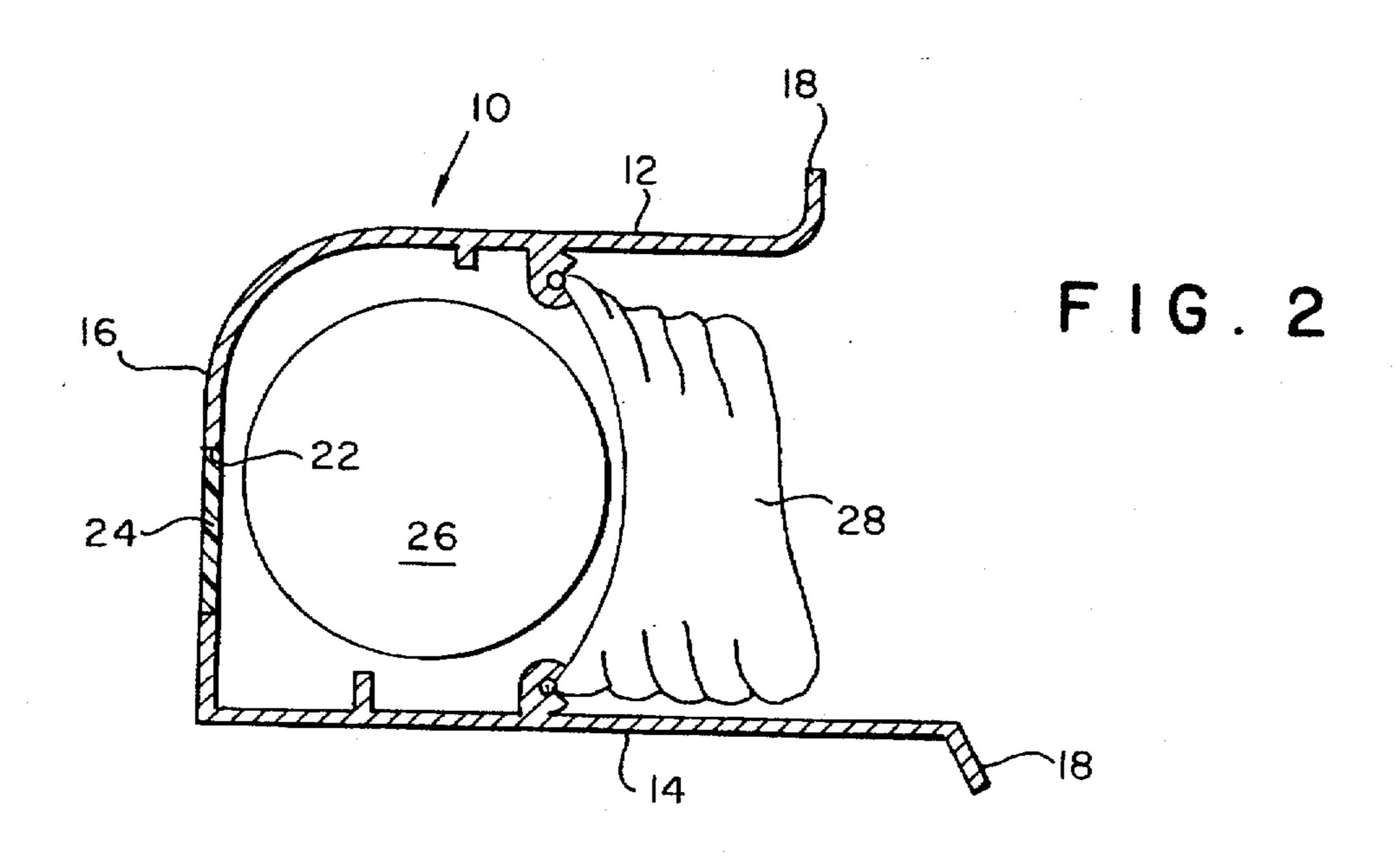
This invention relates to an improvement in the extruded aluminum cans which serve as module housings in passenger side airbag installations. More particularly it relates to a module can with means to avoid pressurization of the can during autoignition when the airbag module can is exposed to bonfire conditions.
