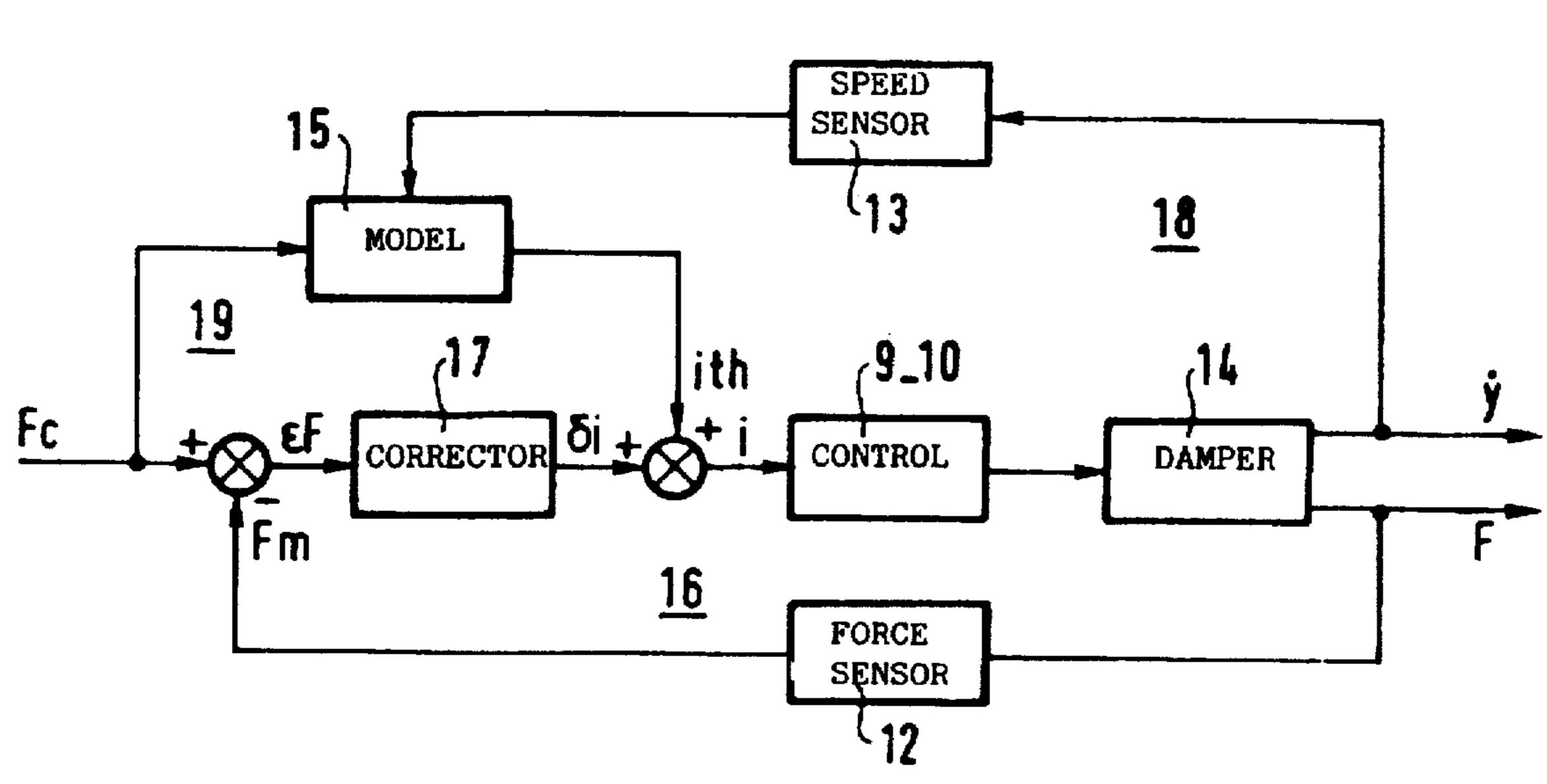
SEMI-ACTIVE SUSPENSION SYSTEM WITH CONTROL CIRCUIT HAVING A DIRECT CONTROL LOOP INCLUDING AN INVERSE
