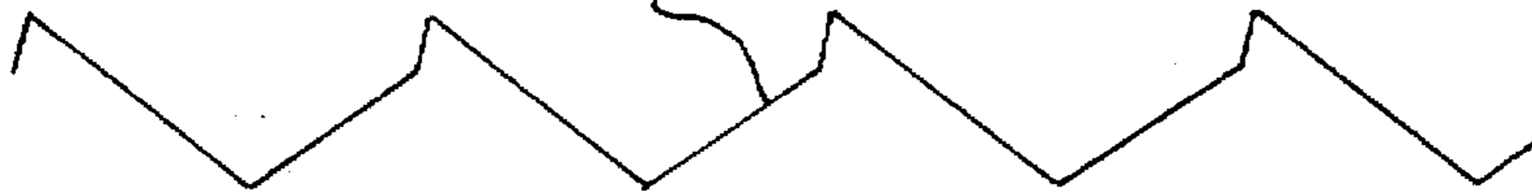
VOLTAGE AT Q OUTPUT OF R-S LATCH 470
