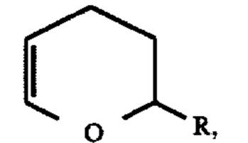
in which R stands for C<sub>1</sub> to C<sub>20</sub> alkoxy, with water at temperatures ranging from 0° to 150° C. and pressures of from 0.01 to 50 bar in the presence of a which microporous, crystalline aluminum silicate catalyst, e.g. a beta-type zeo-lite or pentasil catalyst having a pore diameter greater than 5.4 Å.
