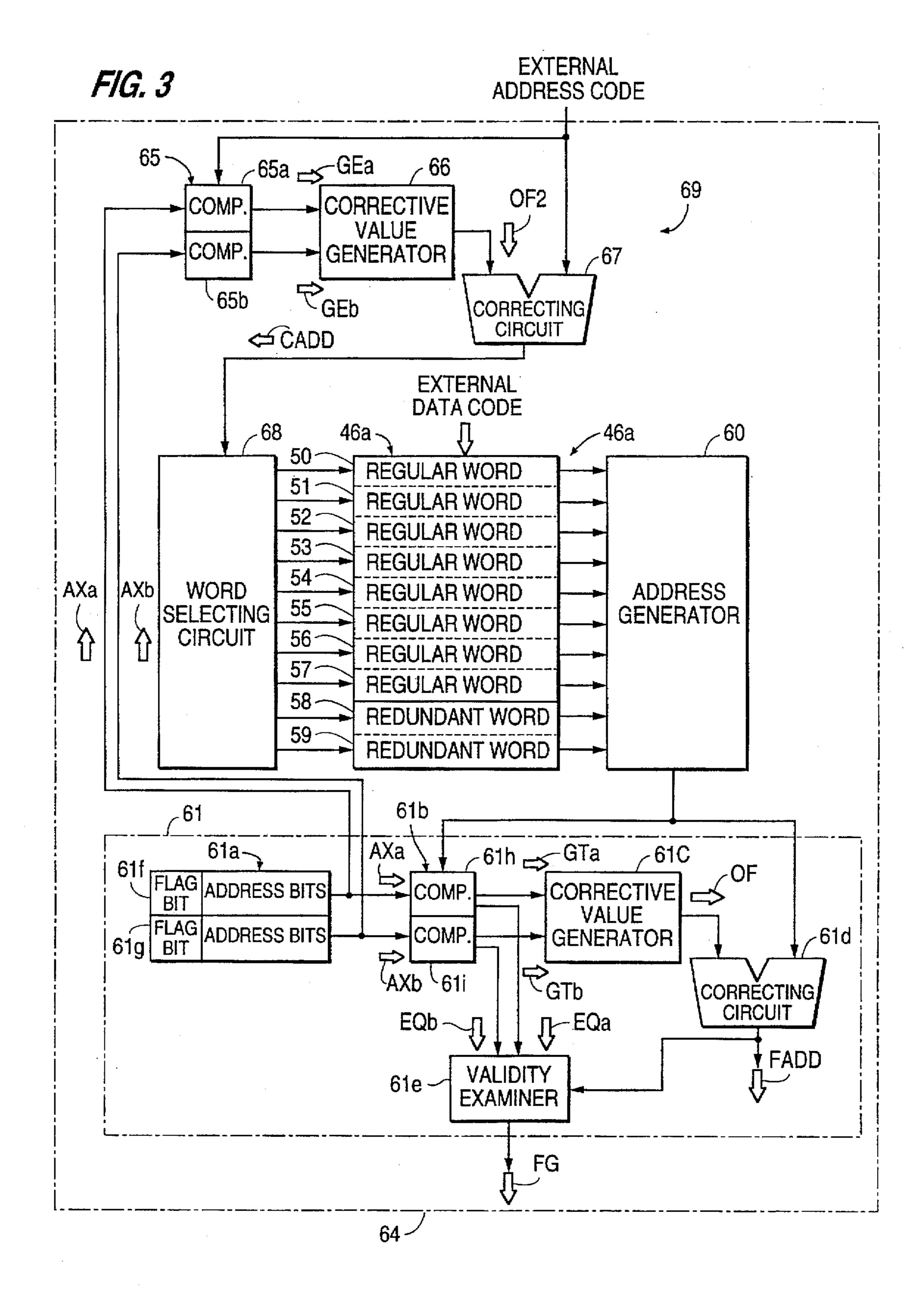
SEMICONDUCTOR ASSOCIATIVE MEMORY DEVICE WITH ADDRESS CORRECTOR FOR GENERATING FORMAL ADDRESS SIGNAL REPRESENTATIVE OF ONE OF REGULAR MEMORY WORDS PARTIALLY REPLACED WITH REDUNDANT MEMORY WORD
