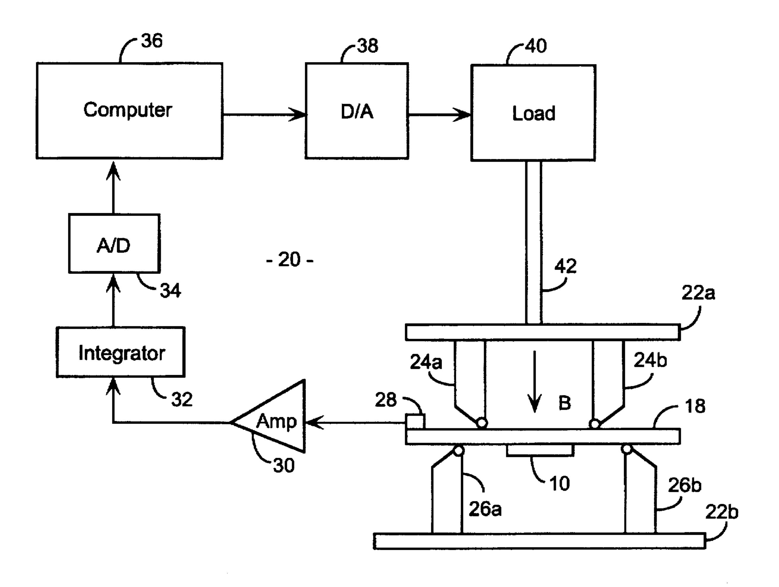
Strain Gauge Test System
