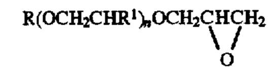
with a salt of a sulfite bisulfite salt mixture at a temperature below about 110° C. wherein R is an alkyl or alkenyl of 10 to 20 carbon atoms, inclusive, R' is hydrogen or methyl and n has an average value of 1 to 10 and obtaining a sulfonated alkoxylated product having as a major quantity of the alkoxylated material a salt of
