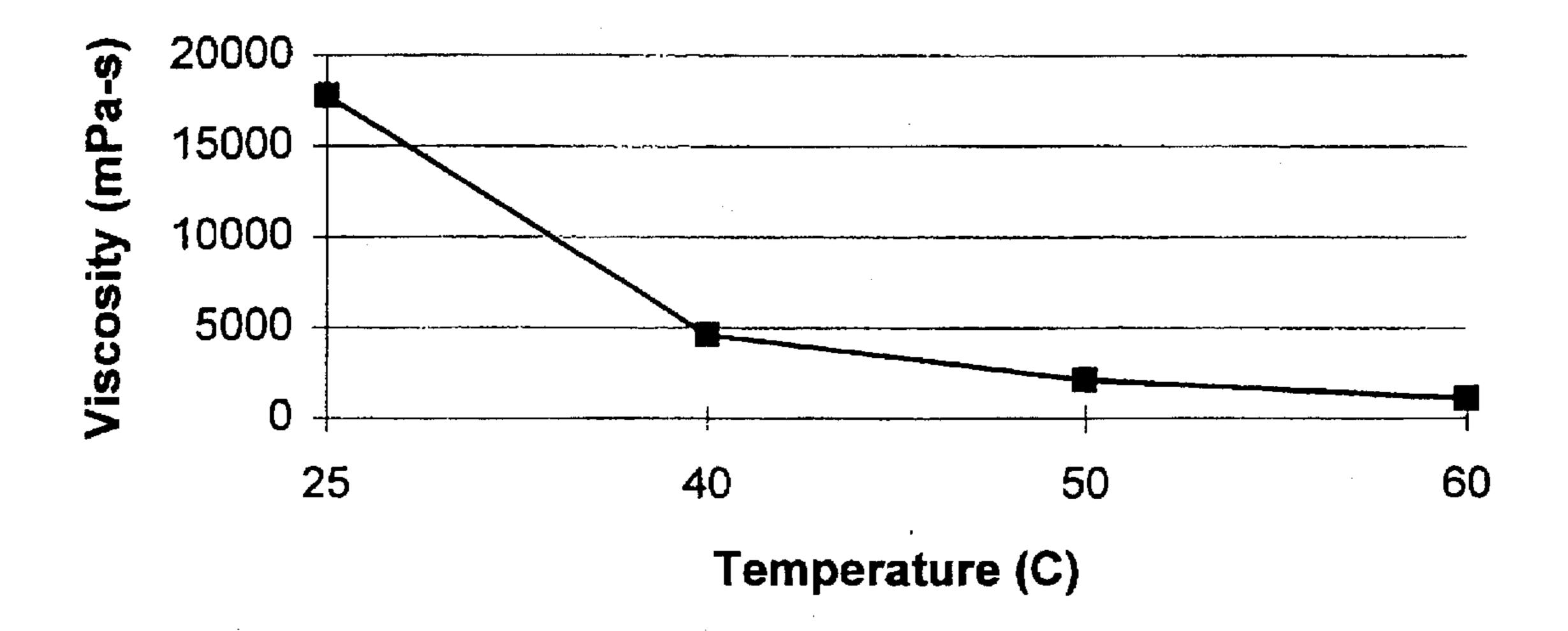
Figure 2: Thermal Profile for Low VOC Pigmented/ Polyol Grind
