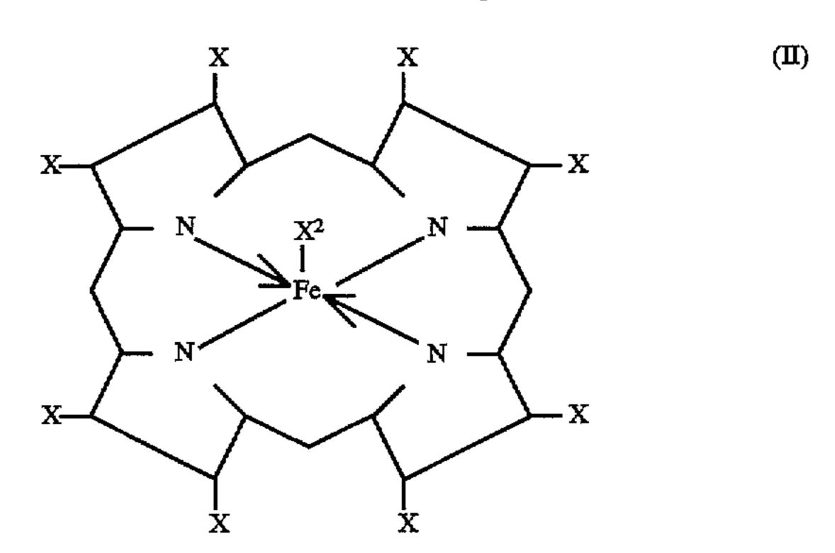
where X can be alkyl, alkyl carboxy, alkyl hydroxyl, vinyl, alkenyl, alkyl sulfate, alkylsulfonate, sulfate, sulfonate.
