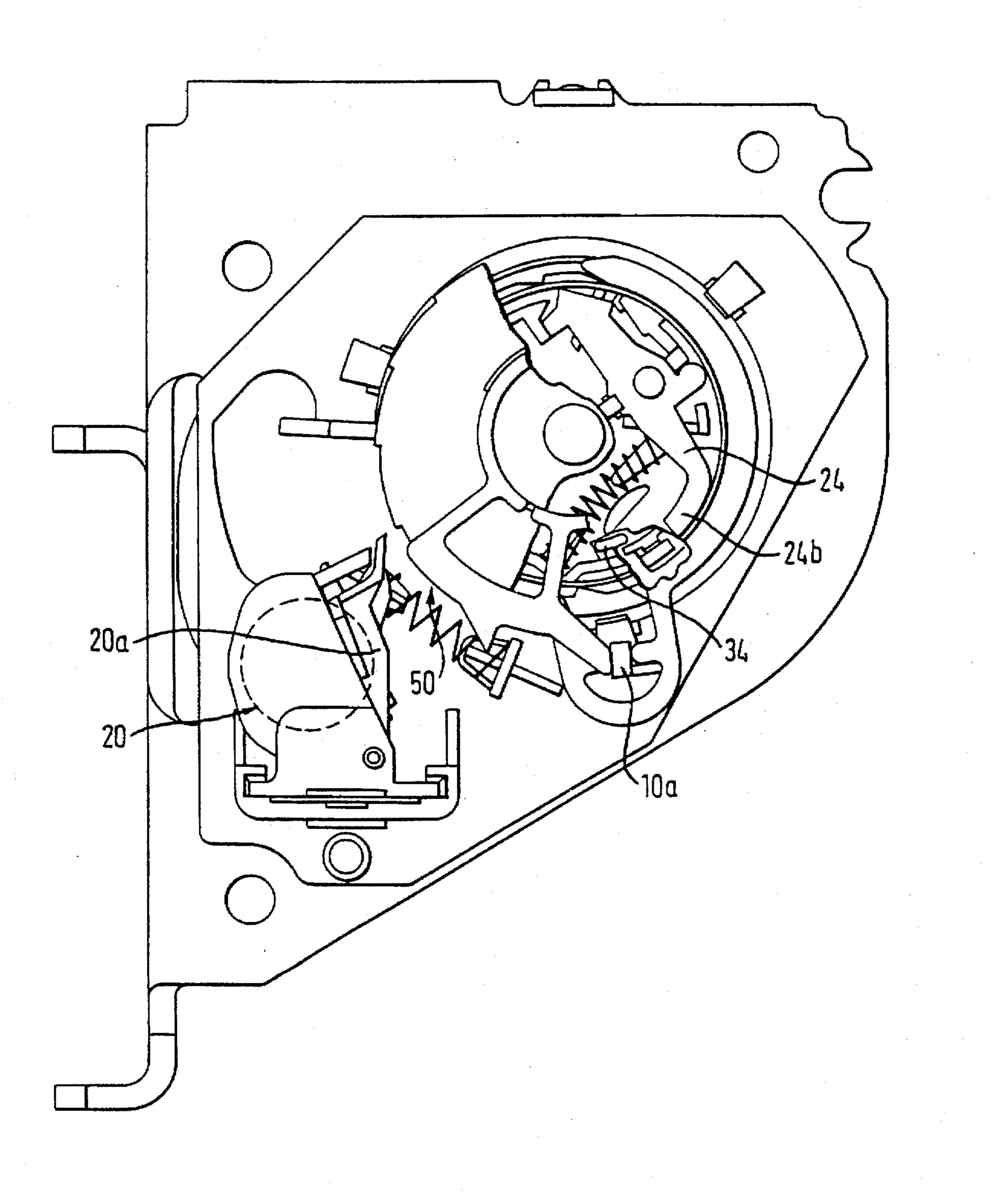
The invention relates to a belt retractor for an occupant restraining system in vehicles comprising a belt drum rotatably mounted in a frame and acted upon by a wind-up spring, a locking mechanism for the belt drum and adapted to be activated by the pivoting, caused in a manner respon-
