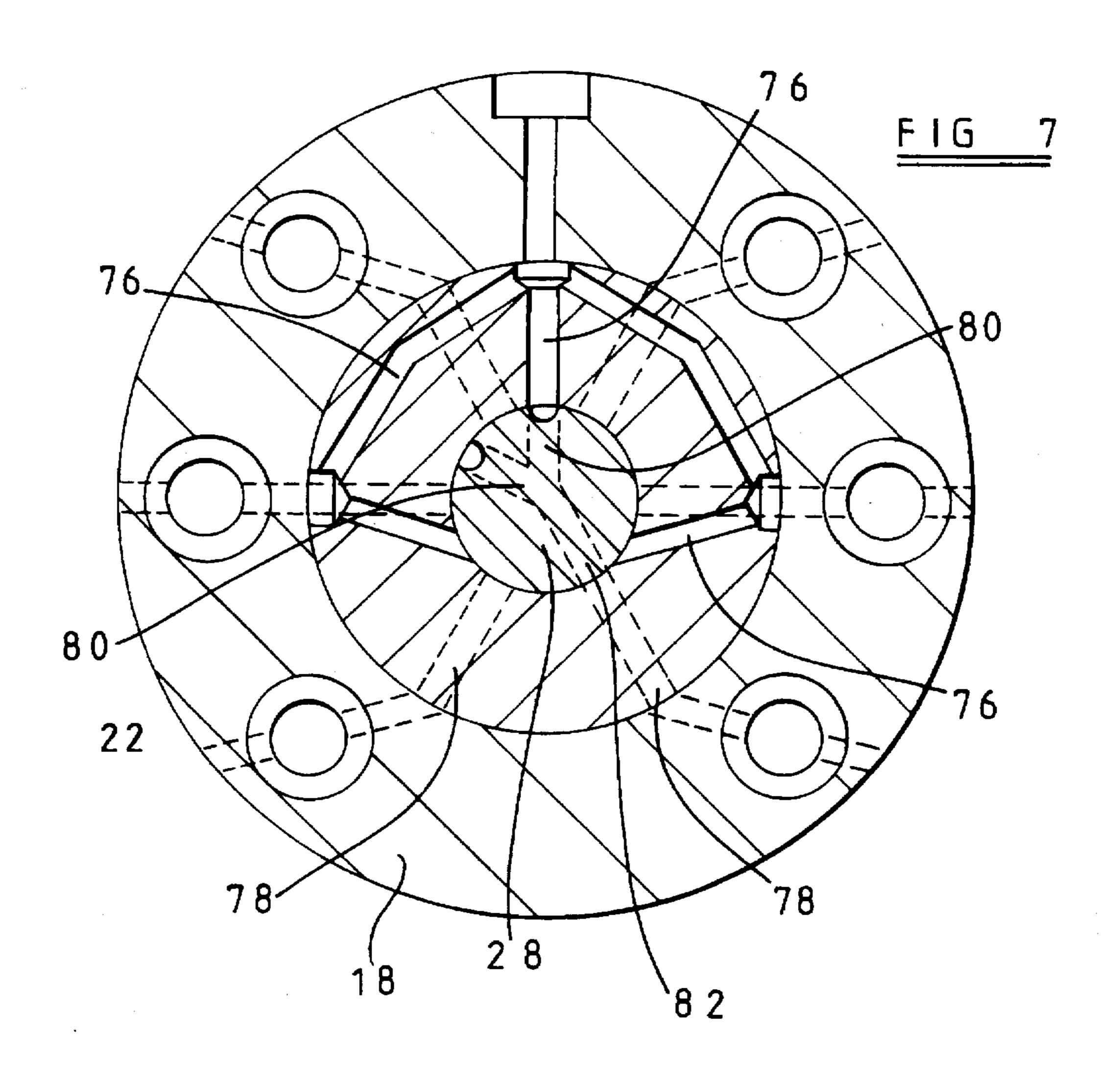
This invention relates to a fuel supply apparatus suitable for use in the supply of fuel to the cylinders of an internal combustion engine, and to a distributor for use in such an apparatus.
