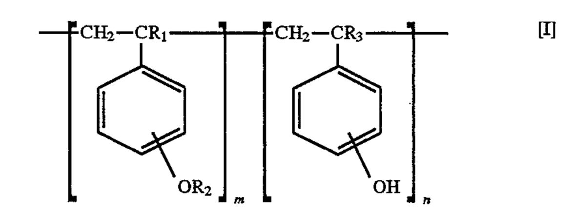
wherein R<sub>1</sub> and R<sub>3</sub> may be the same or different, and represent a hydrogen atom or a methylene group; R<sub>2</sub> represents
