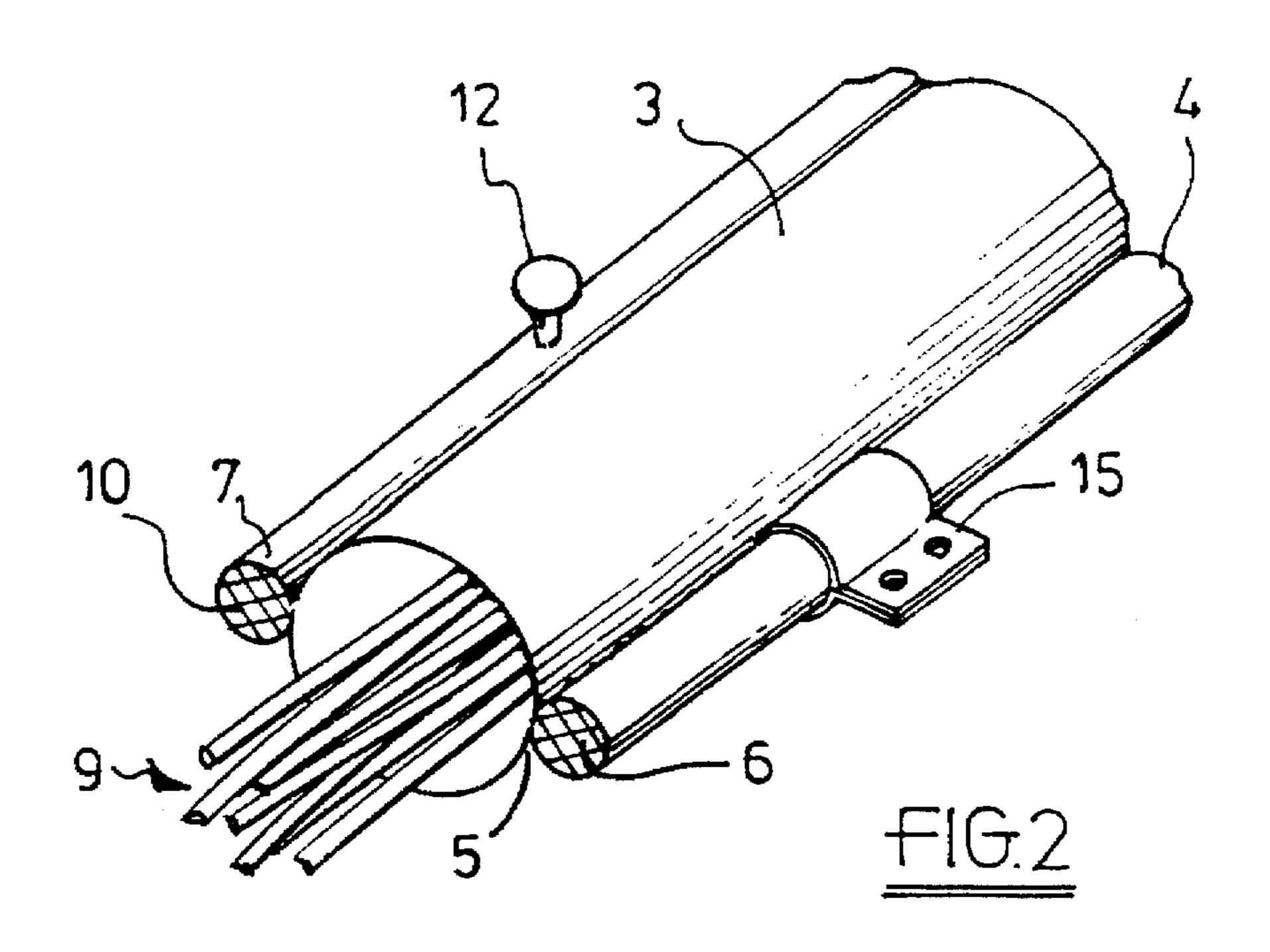
This invention relates to braided textile tubes of the kind commonly used for shielding and/or protecting bundles of wires and/or cables. Such products are typically used to 5 enclose the wiring harness in motor vehicles. The braid
