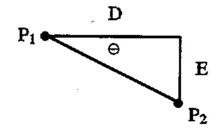
Remember that distances on maps are projected distances. In the FIGURE, D is the (projected) distance between the two points  $P_1$  and  $P_2$ , E is the elevation difference between the points, and  $\theta$  is the pitch of the slope between the two points.
