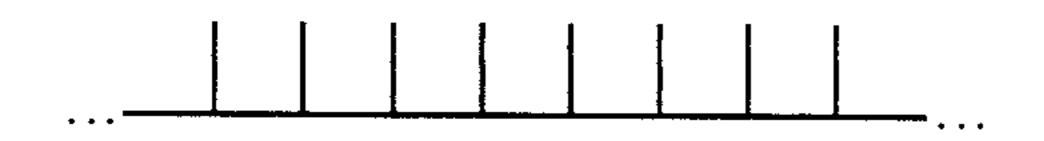
Isotactic polypropylene is capable of being a highly crystalline polymer with a high melting point and other desirable physical properties that are considerably different from the polymer in an amorphous (noncrystalline) state.
