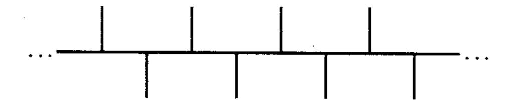
Atactic polymer shows no regular order of repeating unit 45 configurations. In commercial applications, a certain percentage of atactic polymer is typically produced with the crystalline forms.
