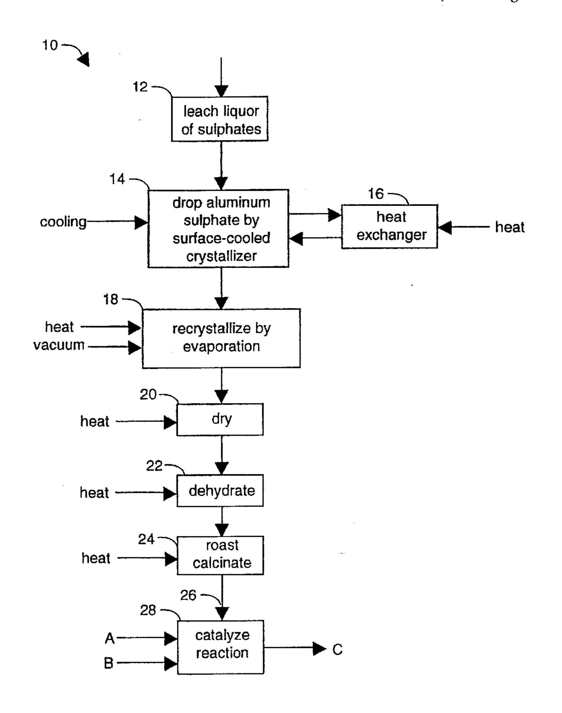
12 leach liquor of sulphates 14 ~ 16drop aluminum heat sulphate by cooling heat exchanger surface-cooled crystallizer 18 recrystallize by heat evaporation vacuum 20dry heat 22dehydrate heat 24 roast heat calcinate 26 28 ~ catalyze reaction B
