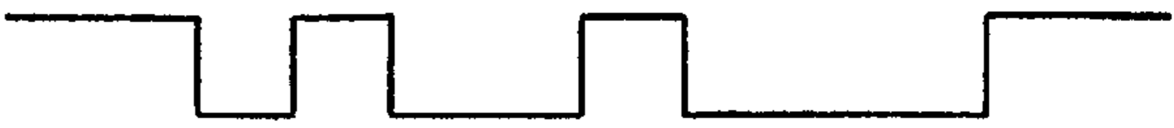
FIG. 21(c) GATE VOLTAGE OF TRANSISTOR T 2
