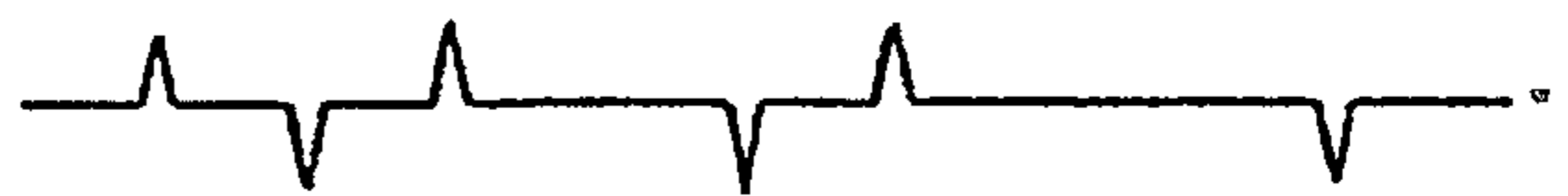
FIG. 13(e) CURRENT FLOWING THROUGH RESISTOR R p
