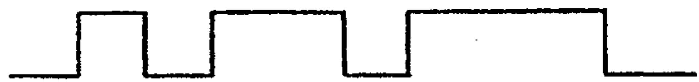
FIG. 13(b) GATE VOLTAGE OF TRANSISTOR T 1
