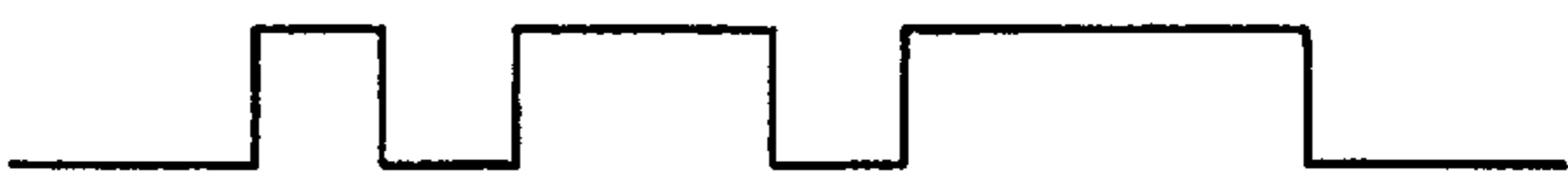
FIG. 21(b) GATE VOLTAGE OF TRANSISTOR T 1
