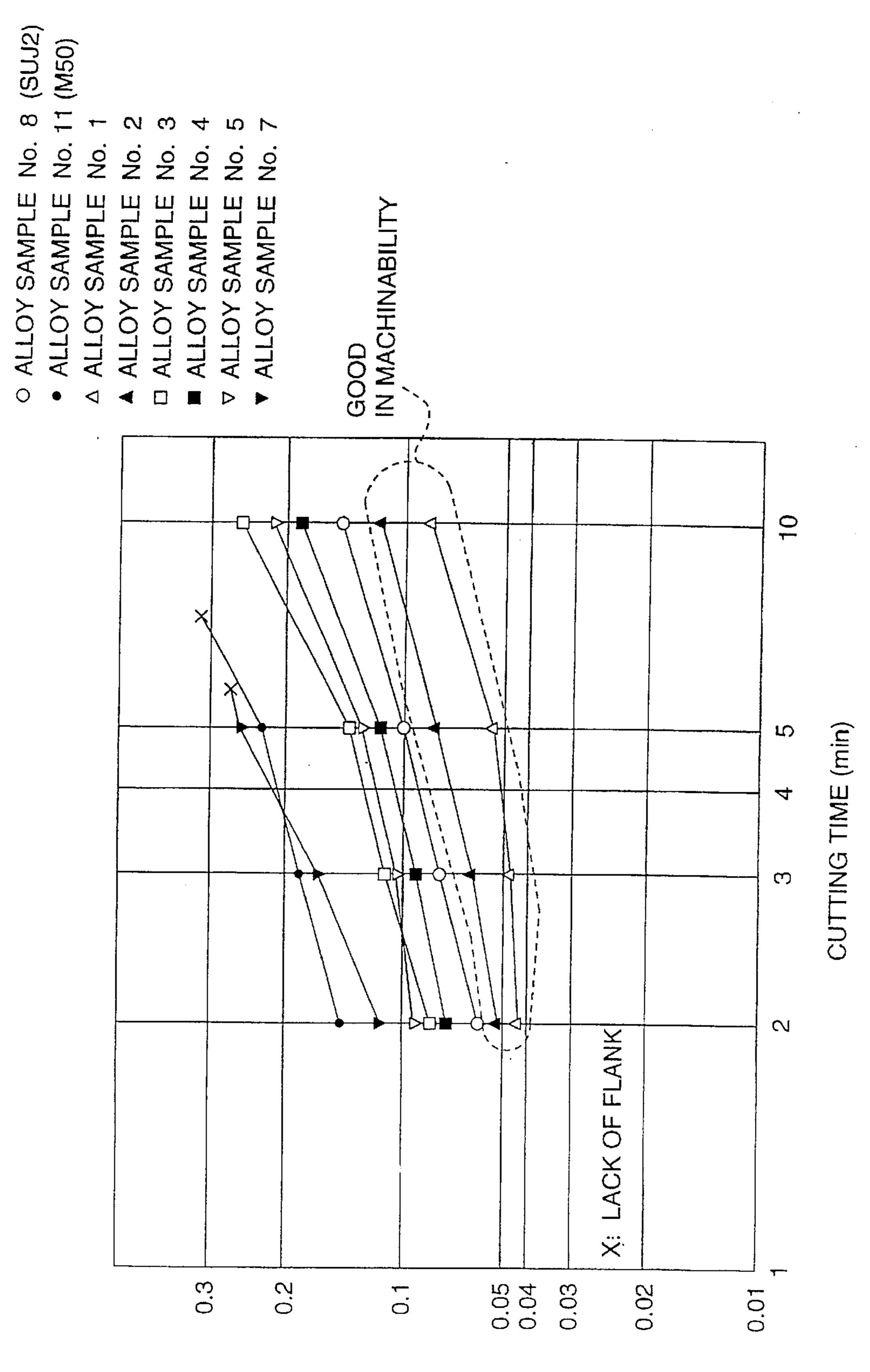
AMOUNT OF WEAR ON A FLANK OF A SINGLE POINT TOOL (mm)
