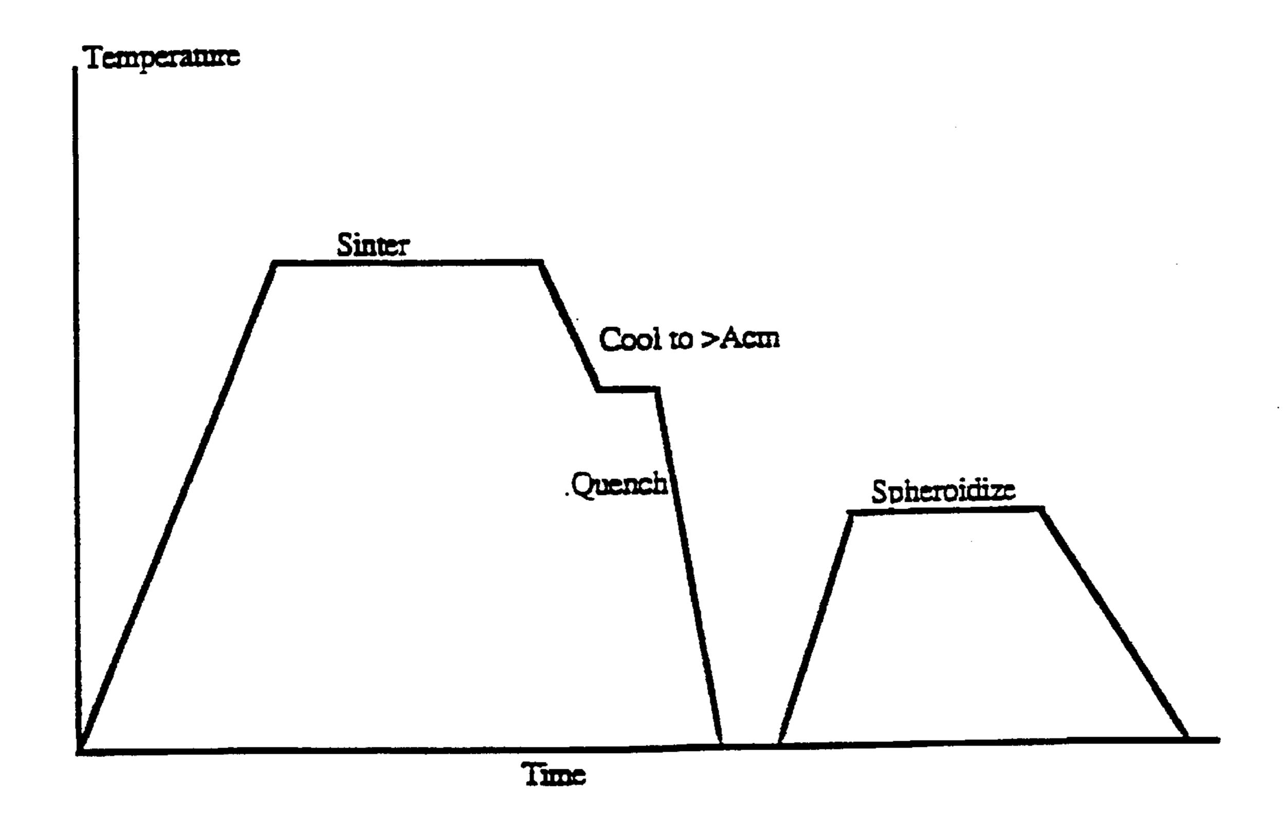
UHCS High Density Powder Metal Process Stages - Schematic Diagram
