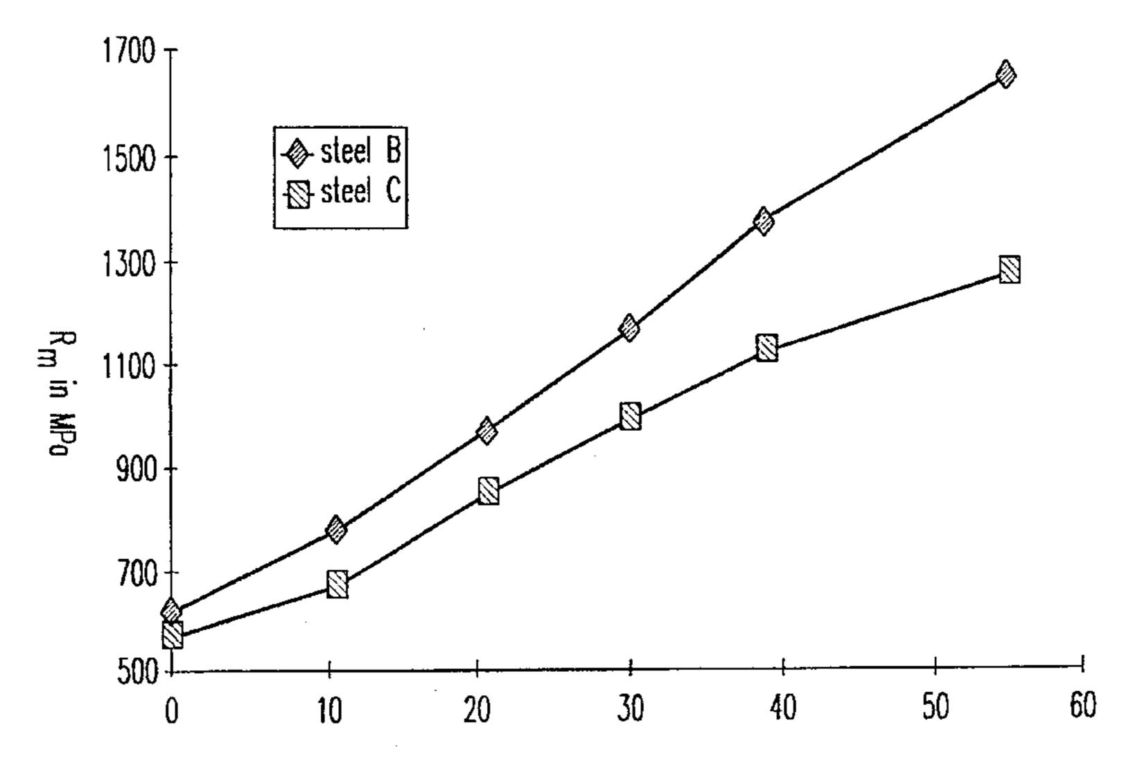
REDUCTION IN CROSS SECTION BY WIRE-DRAWING, IN %
