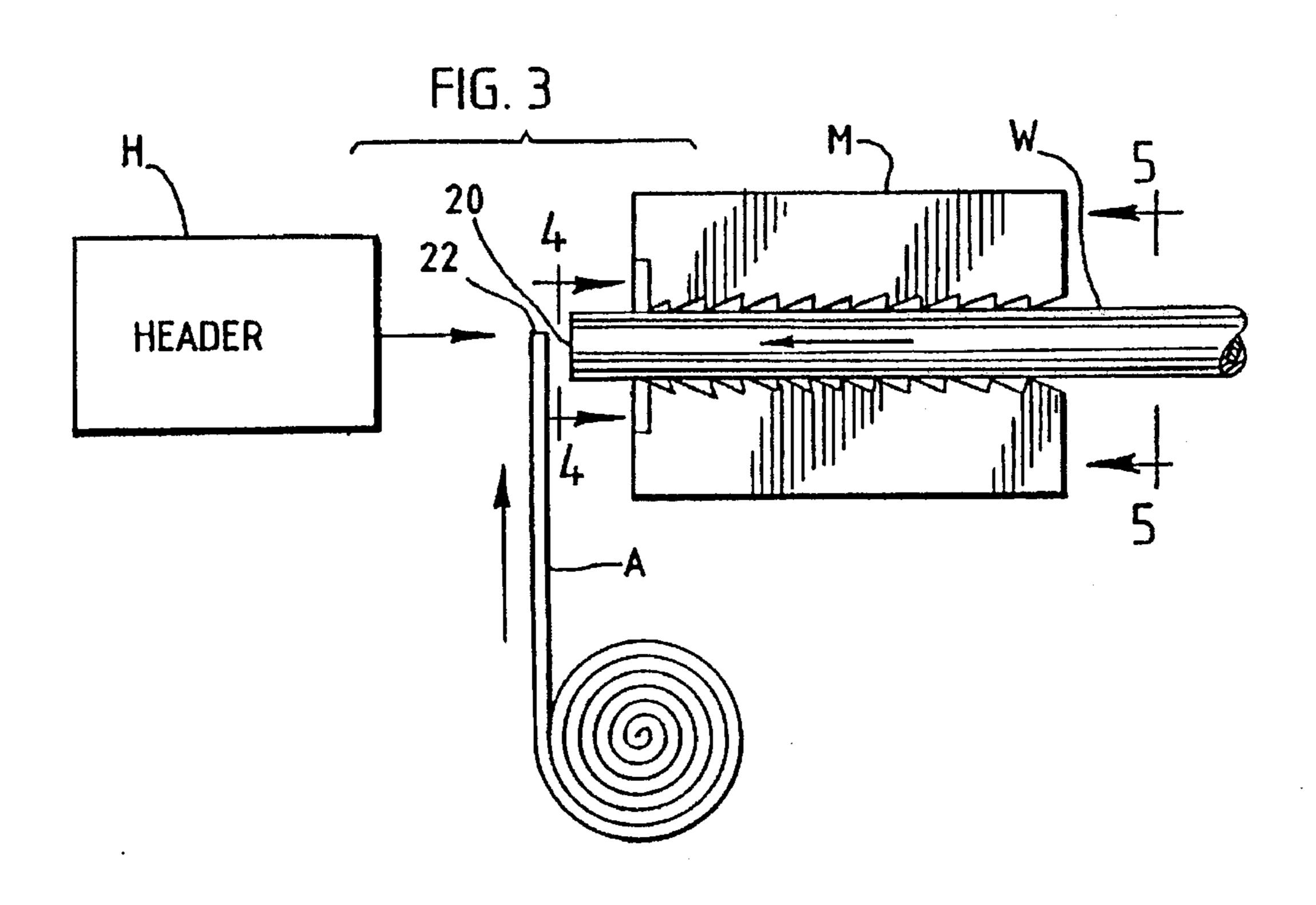
METHOD OF MANUFACTURING A CORROSION-RESISTANT, HEADED FASTENER, SUCH AS NAIL FOR EXTERIOR APPLICATIONS, AND MANUFACTURING METHOD
