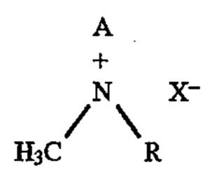
where R is methyl or ethyl; X is the anion of an inorganic or organic, but not phytotoxic acid, preferably bromide or chloride, and A is a chain of 4 or 5 methylene groups, which chain may be substituted by chloro, bromo, methyl, cholormethyl, bromomethyl, hydroxymethyl, and methylene, or which chain containing one or two double bonds, or A is the chain —(CH<sub>2</sub>)<sub>n</sub>—NH—, where n is 3 or 4, disclosed in U.S. Pat. No. 3,905,798 and hereby incorporated by reference.
