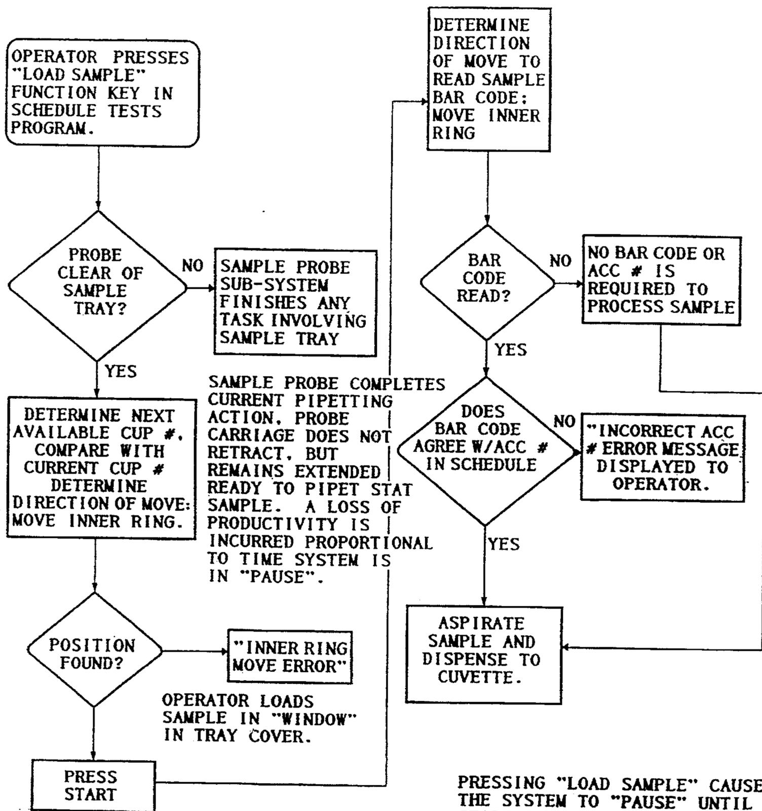
PRESSING "LOAD SAMPLE" CAUSES THE SYSTEM TO "PAUSE" UNTIL START IS PRESSED TO RESUME OPERATION. SAMPLES IN PROCESS CONTINUE TOWARD COMPLETION.
