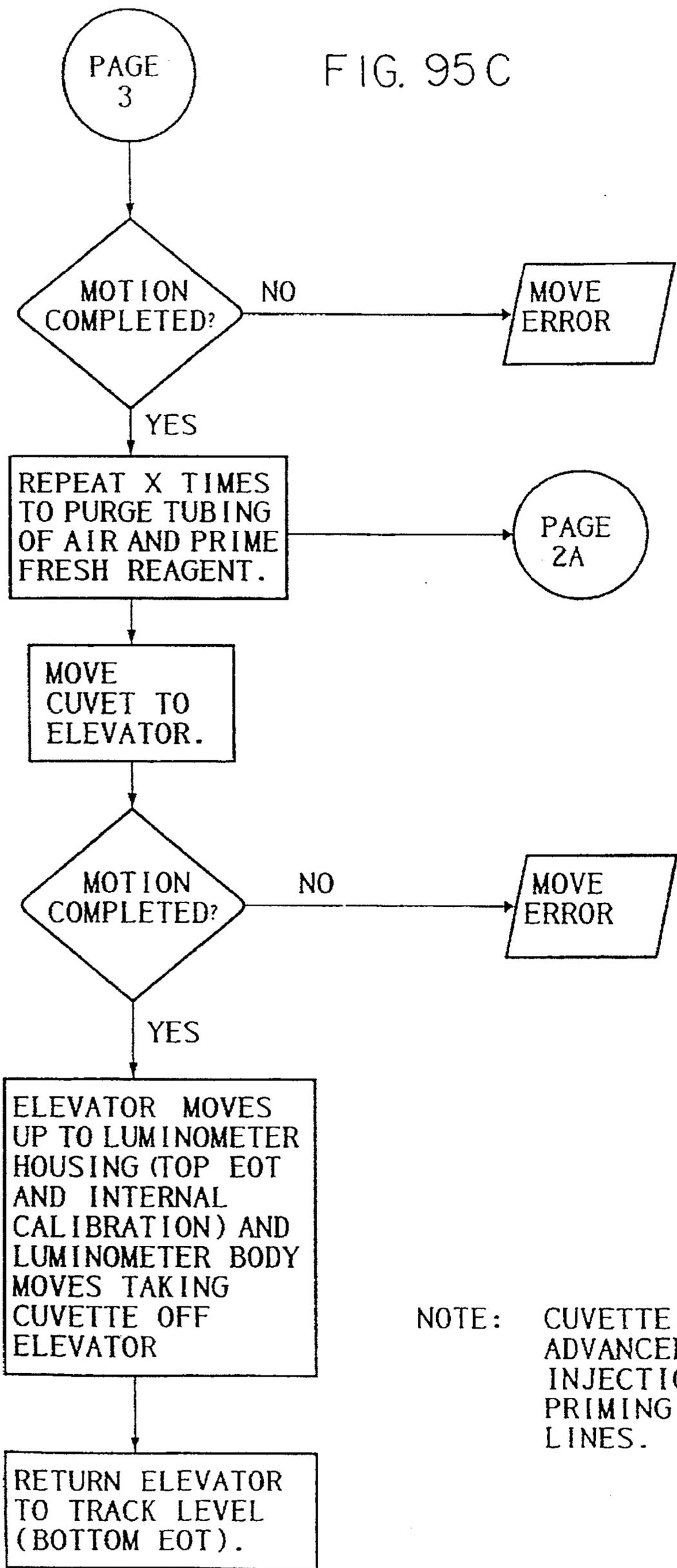
NOTE: CUVETTE IN LUMINOMETER IS ADVANCED TO PMT/BASE INJECTION POSITION FOR PRIMING THE BASE REAGENT LINES.
