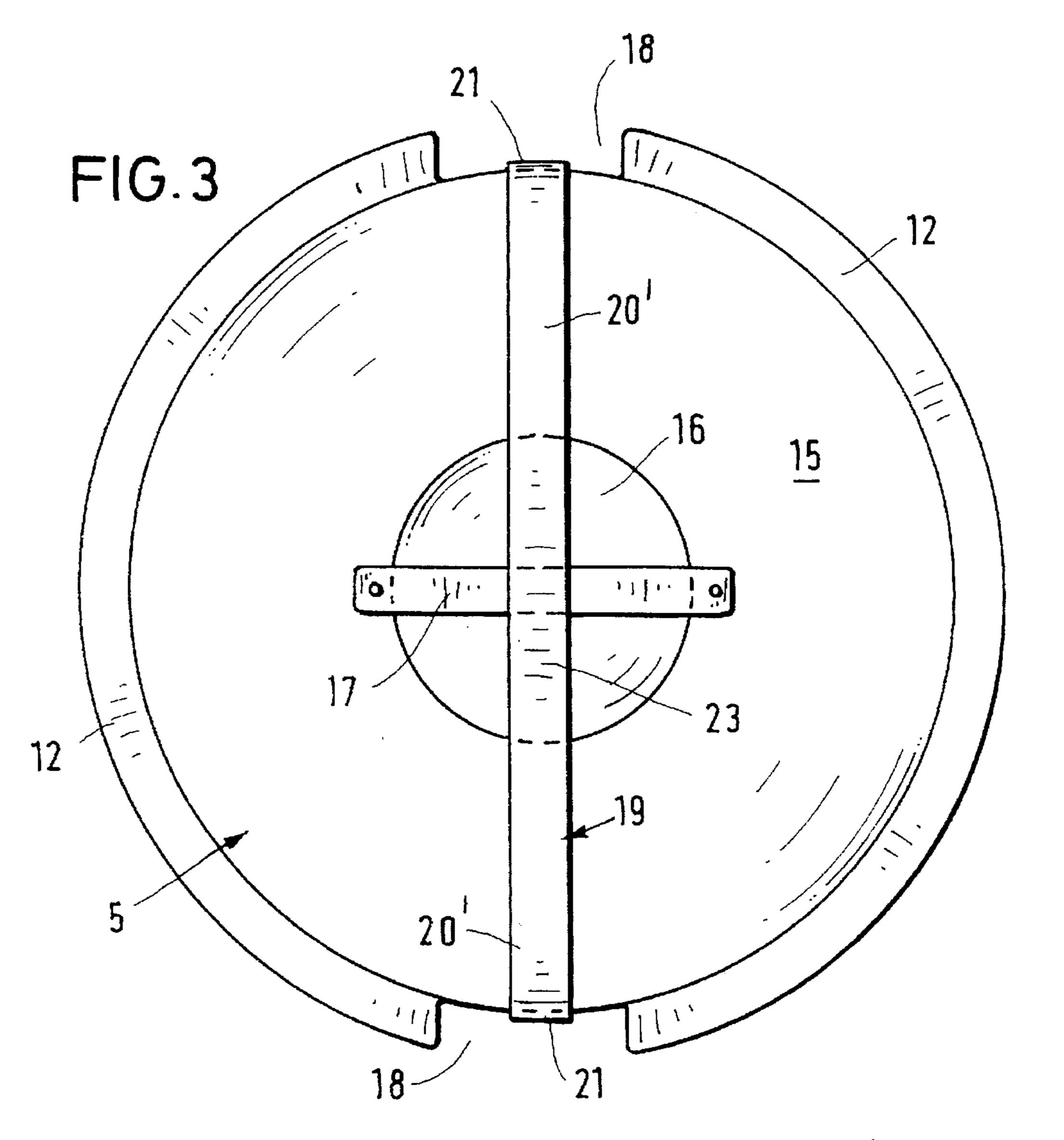
The invention relates to a springform with a clampable form rim arranged detachably on the form bottom and provided with a clamping closure, and with a covering hood which can be mounted on the form bottom.
