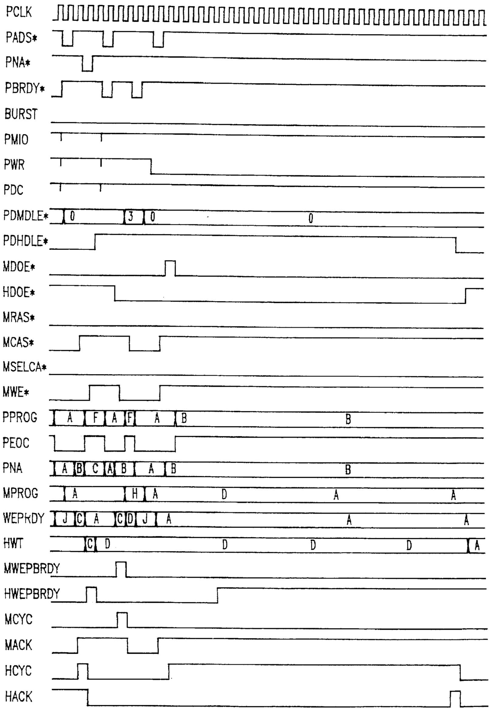
HOST WRITE/MEMORY WRITE, FULLY PIPELINED
