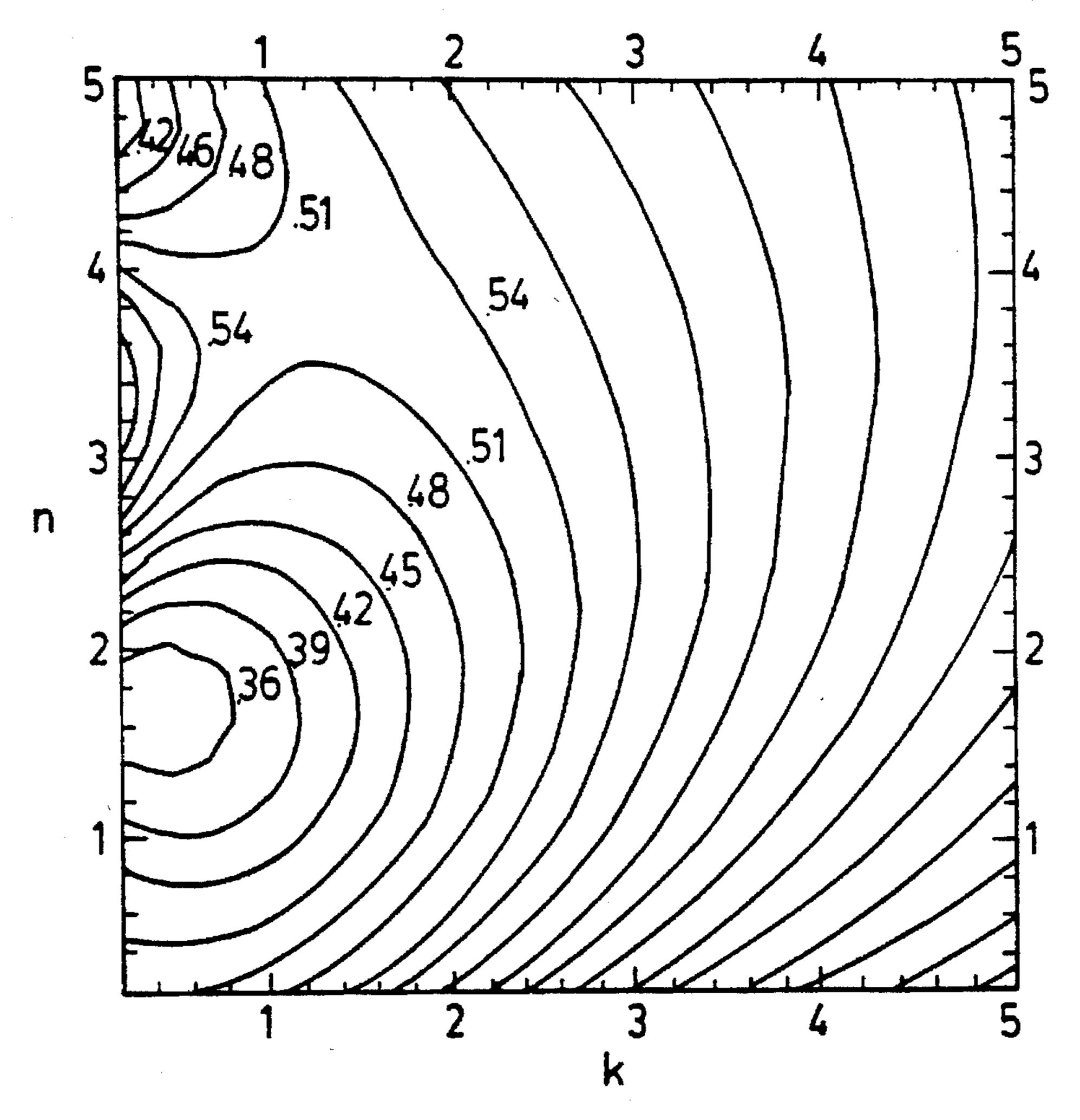
$\lambda = 248 \, \text{nm}$ XP8843 / ARL / W-Si  $n_{PR} = 1.802$ ,  $k_{PR} = 0.0107$ ,  $d_{PR} = 1.0 \mu m$ nari, kari: parameter, dari=0.03 µm nsub = 1.96, ksub = 2.69
