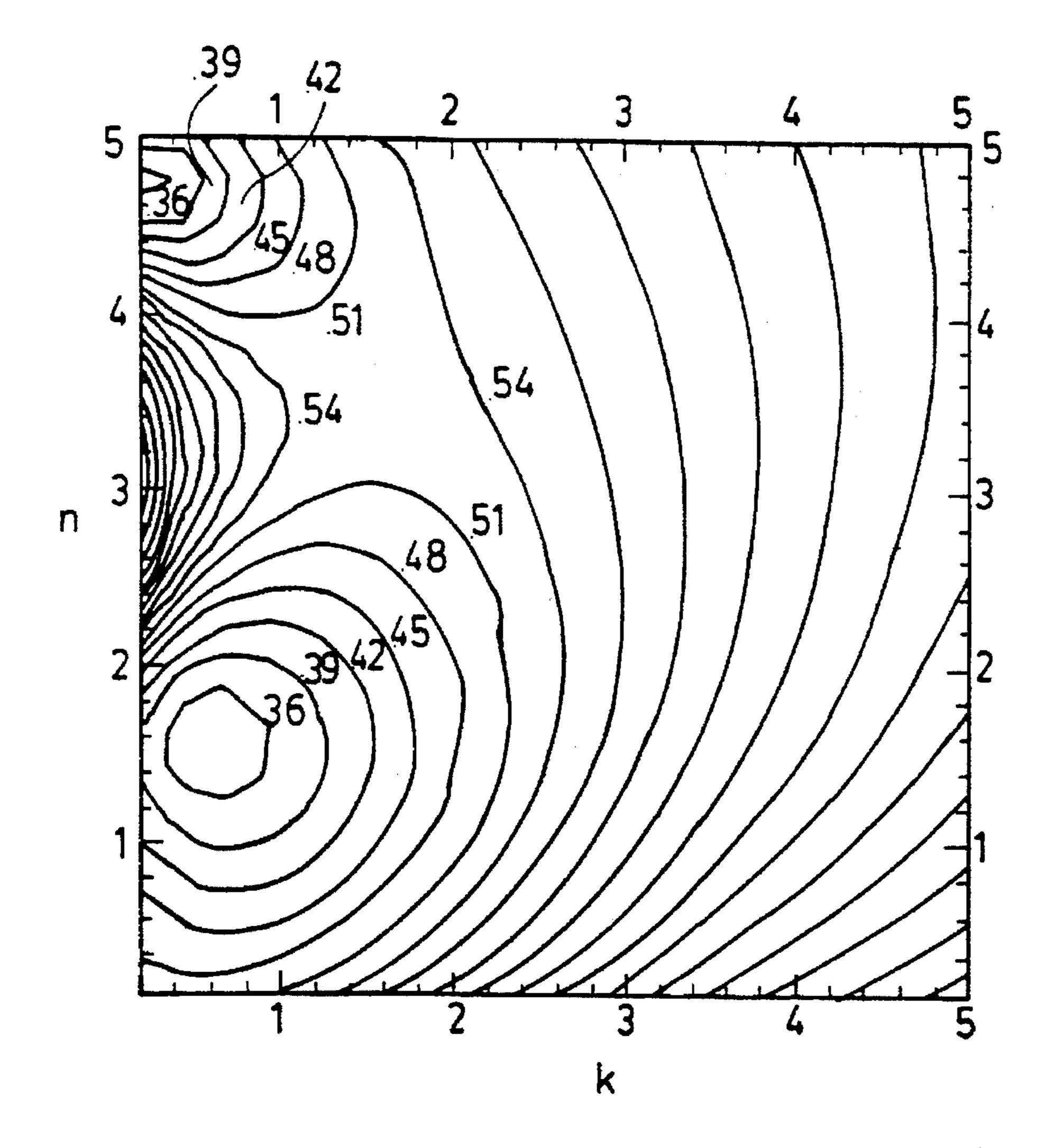
λ=248 nm XP8843 / ARL / AI, AI-Si, AI-Si-Cu, npR=1.802, kpR=0.0107, dpR=1000 nm, nari, kari: parameter, dari=30 nm, nsub=0.089, ksub=2.354
