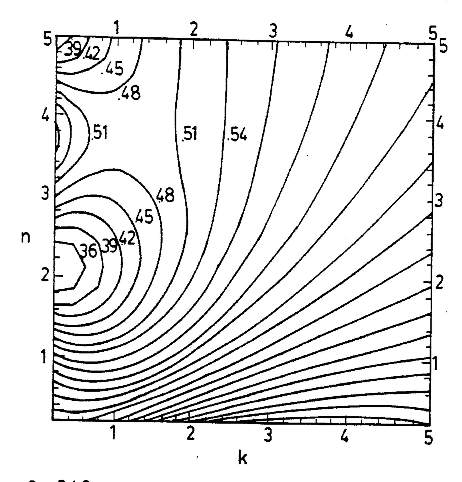
λ=248nm XP8843/ARL/W-Si n<sub>PR</sub>=1.802, k<sub>PR</sub>=0.0107, d<sub>PR</sub>=0.985μm n<sub>arl</sub>, k<sub>arl</sub>: parameter, d<sub>arl</sub>=0.03μm n<sub>sub</sub>=1.96, k<sub>sub</sub>=2.69
