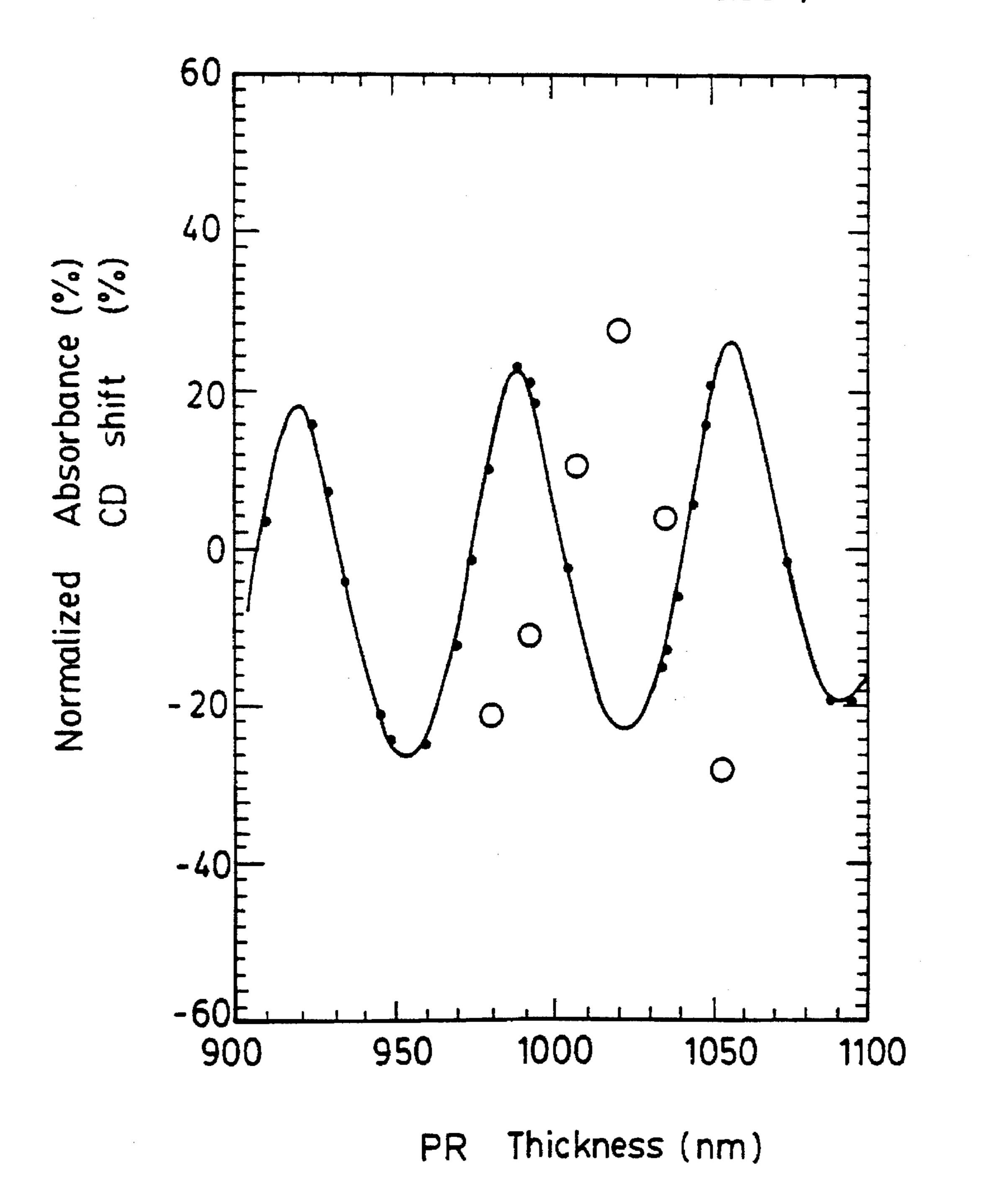
Relation between fluctuation for the amount of absorbed light and dimensional change of pattern
