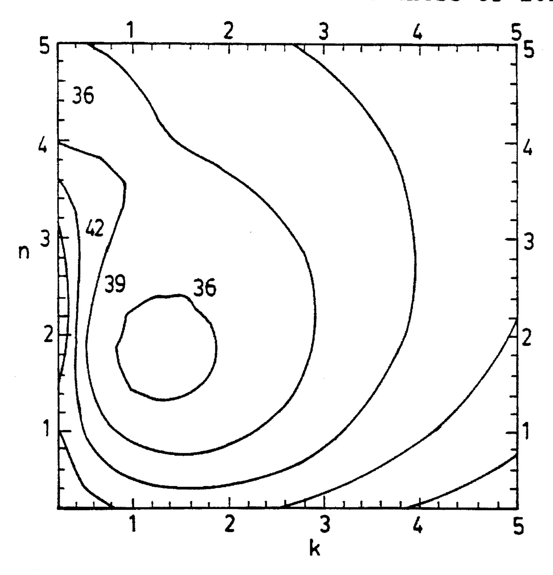
λ=248 nm XP8843 / ARL / W-Si n<sub>PR</sub>=1.802 , k<sub>PR</sub>=0.0107 , d<sub>PR</sub>=1.0175 μm n<sub>arl</sub> , k<sub>arl</sub> : parameter , d<sub>arl</sub>=0.03 μm n<sub>sub</sub>=1.96 , k<sub>sub</sub>=2.69
