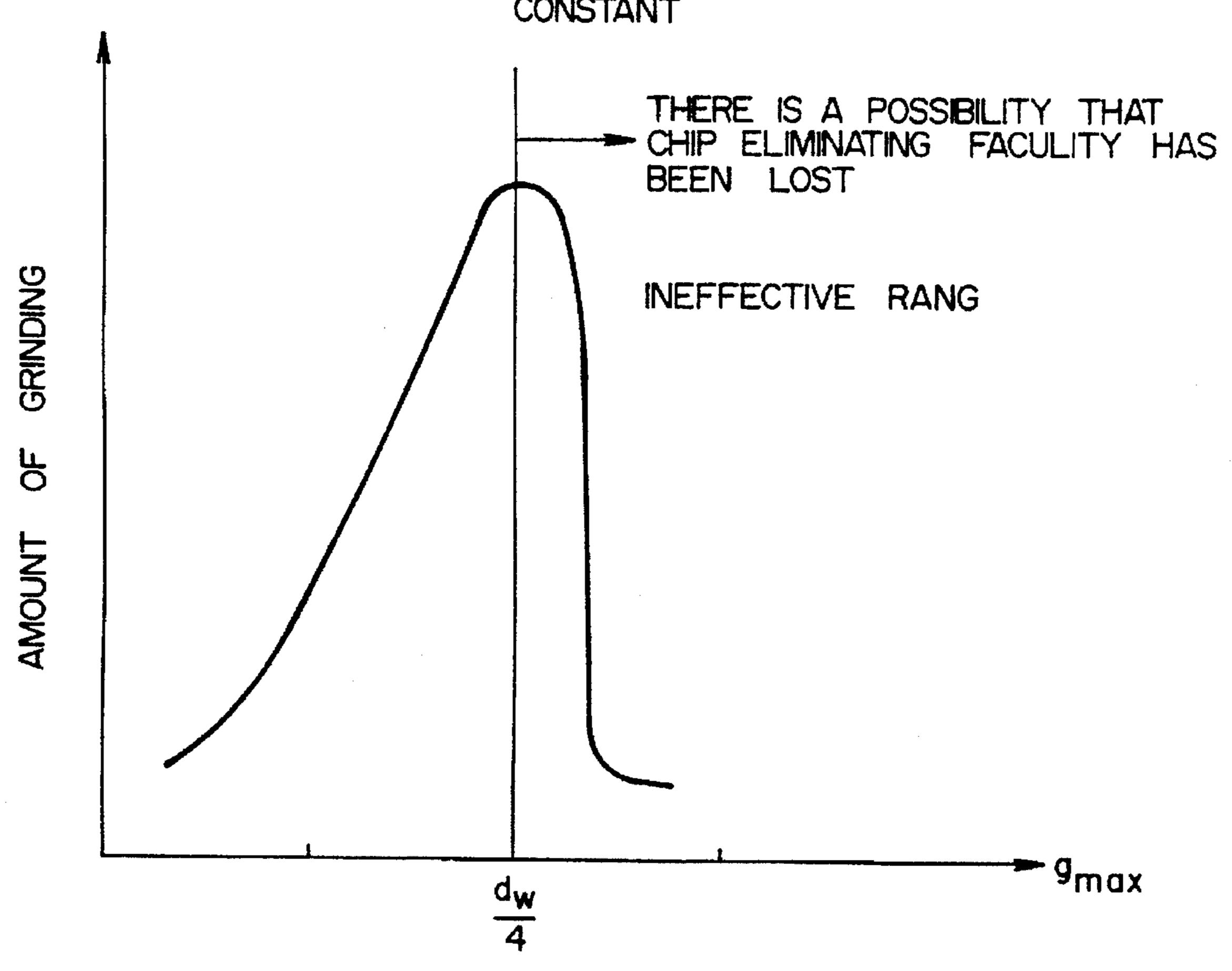
MAXIMUM CUTTING DEPTH OF ONE ABRASIVE GRAIN
