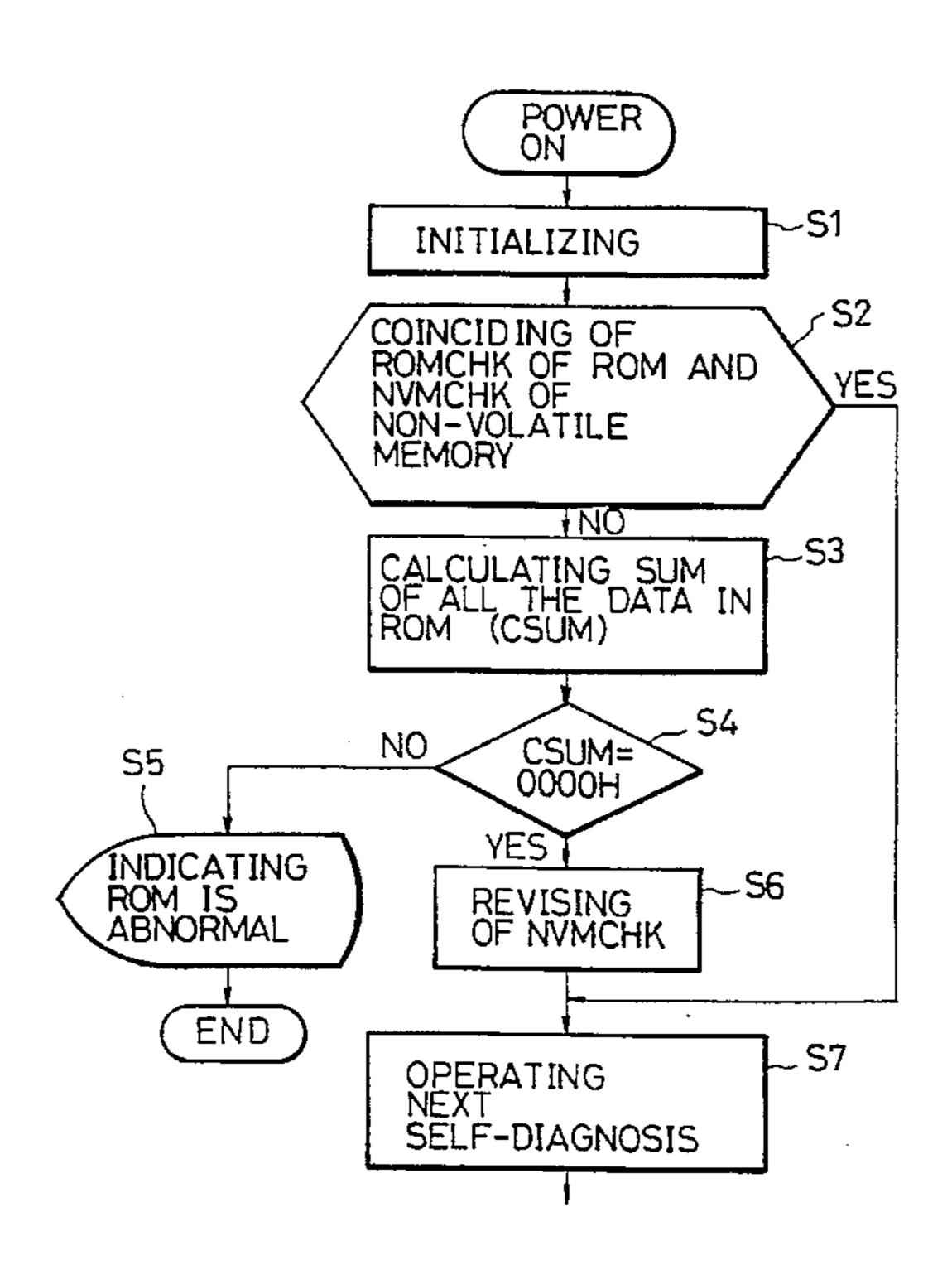
FIG. 1 INITIALIZING COINCIDING OF ROMCHK OF ROM AND NVMCHK OF NON-VOLATILE MEMORY YES ~S3 CALCULATING SUM OF ALL THE DATA ROM (CSUM) ROM **S4** NO CSUM= 000H **S5** YES INDICATING ROM IS ABNORMAL **-**S6 REVISING OF NVMCHK END OPERATING NEXT SELF-DIAGNOSIS
