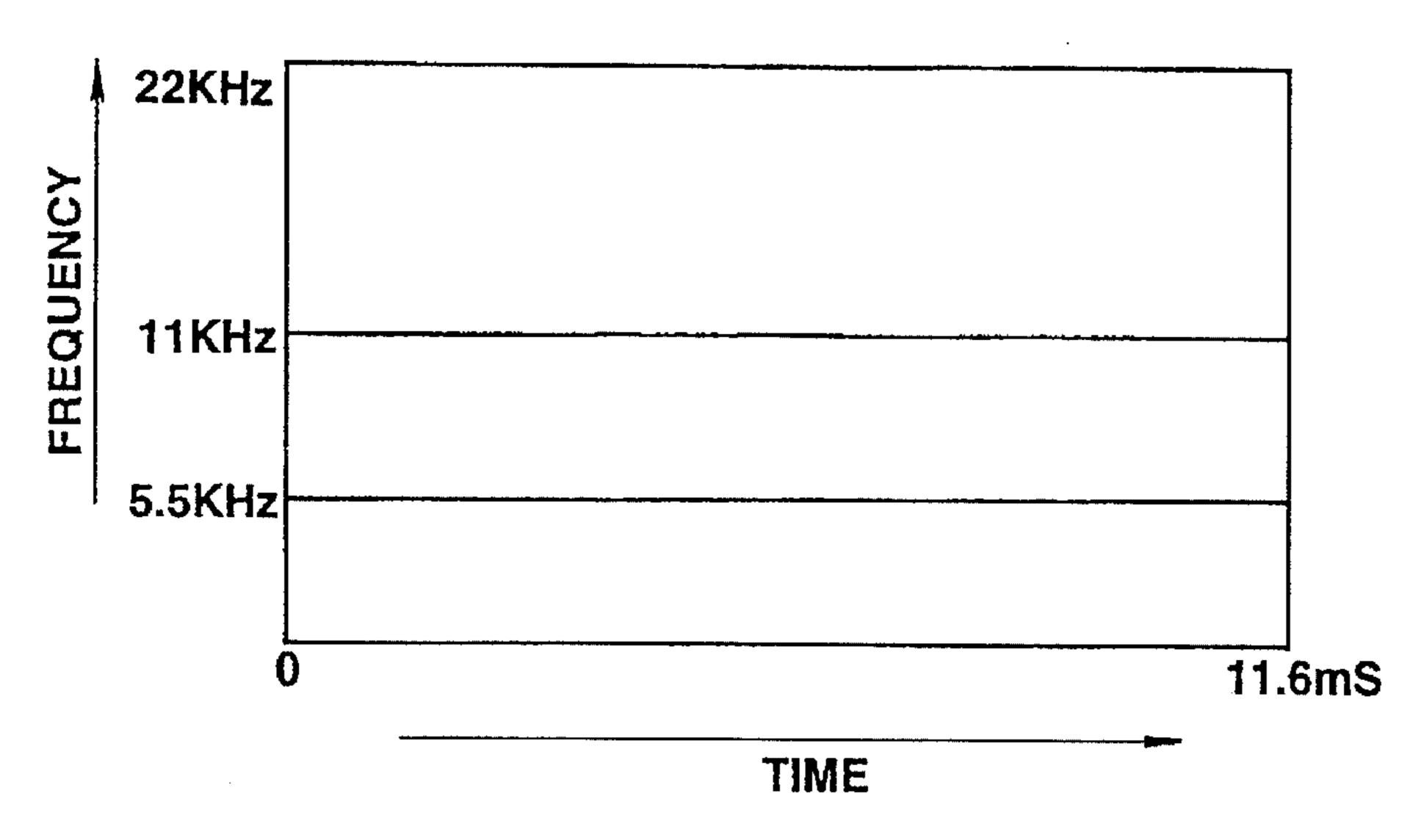
BLOCK SIZE FOR ORTHOGONAL TRANSFORM IN LONG MODE
