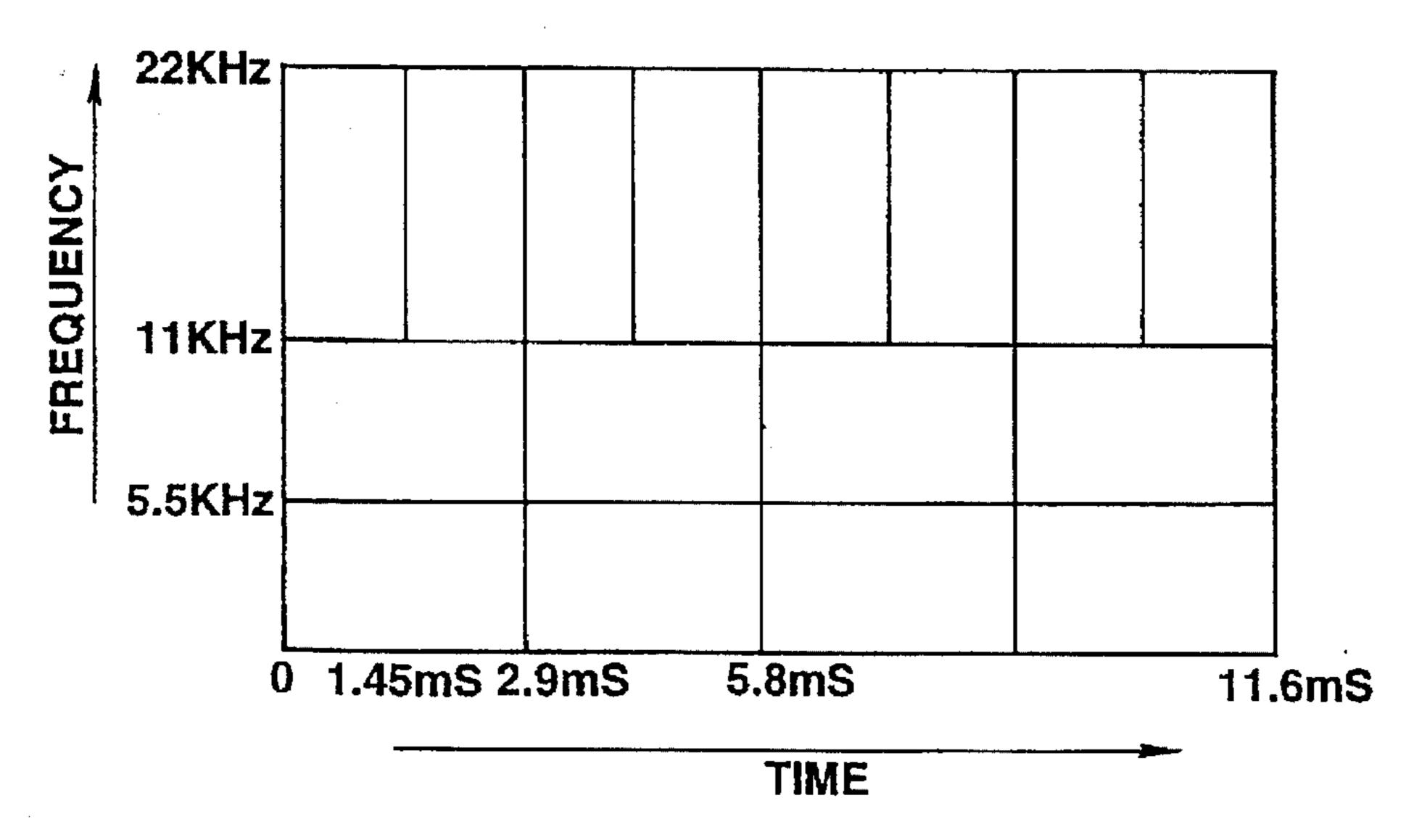
BLOCK SIZE FOR ORTHOGONAL TRANSFORM IN SHORT MODE
