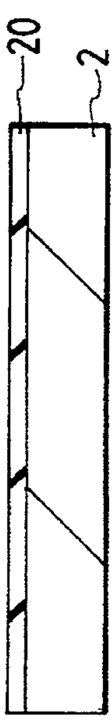
FIG. 16(a) DEPOSITION OF INSULATING FILM
