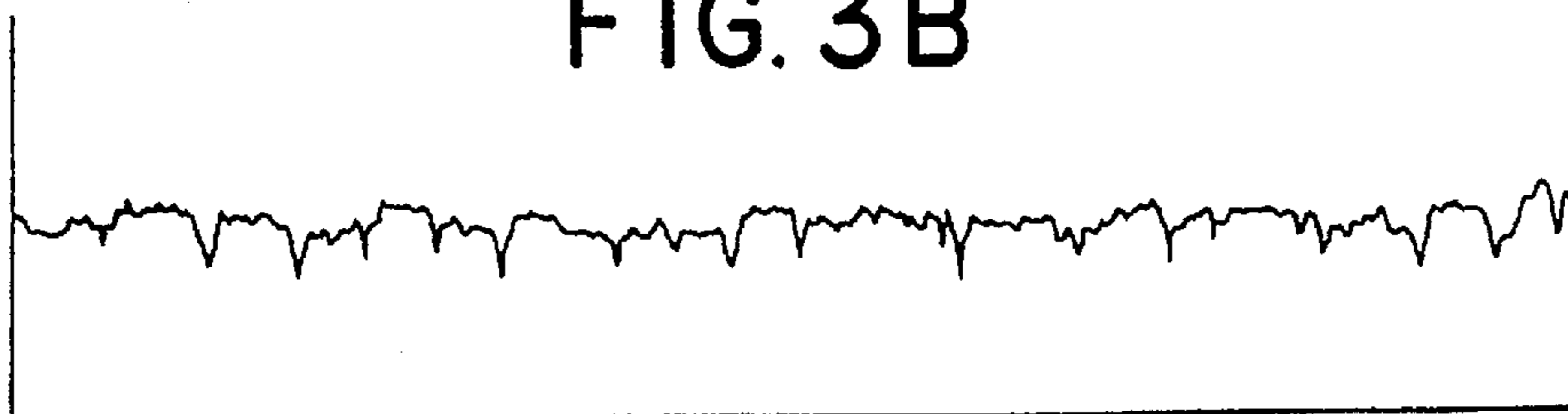
EXAMPLE OF MEASUREMENT OF SURFACE ROUGHNESS (IN THE CIRCUMFERENTIAL DIRECTION)
