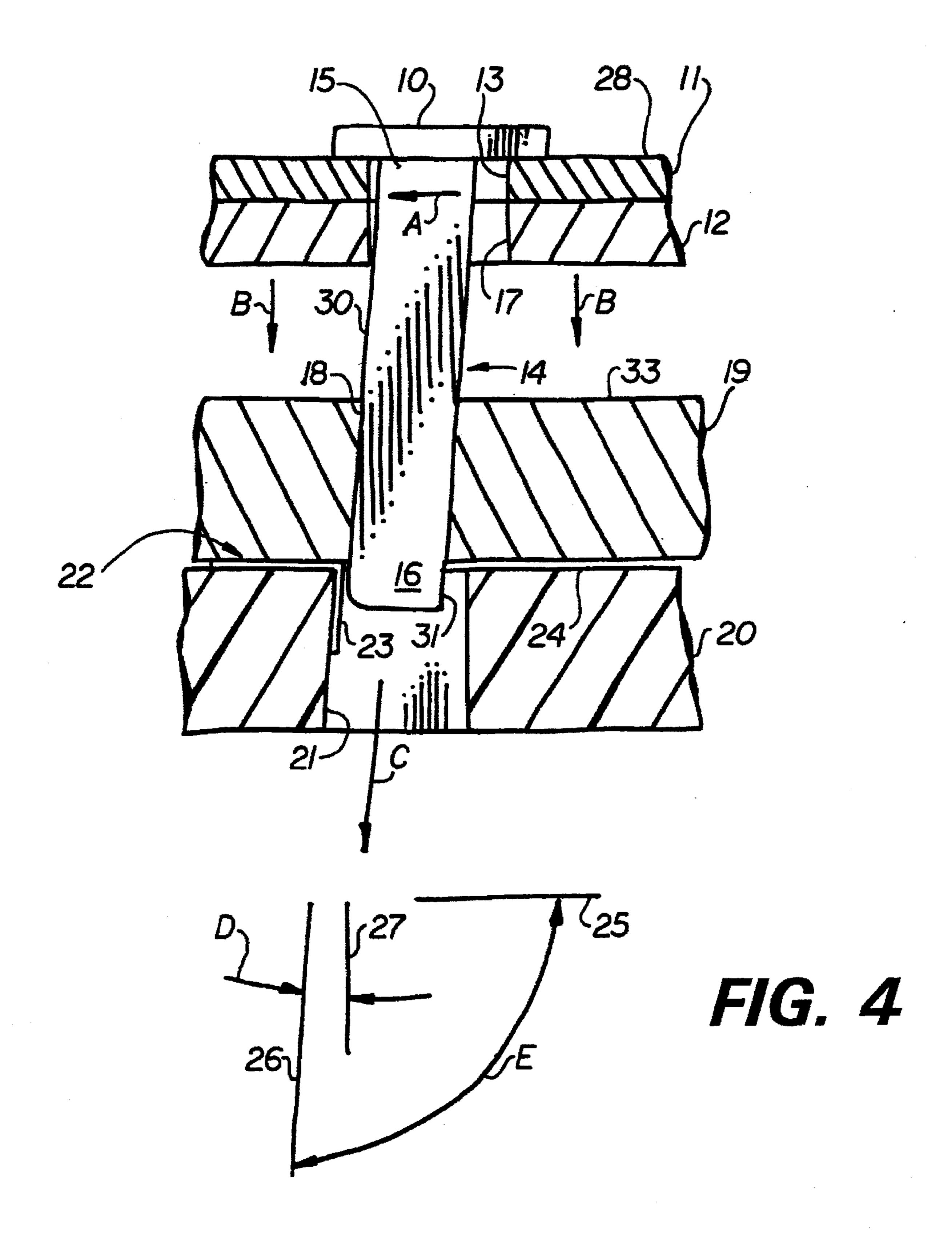
deforming a sheet of material. More particularly, the invention pertains to a punch and
