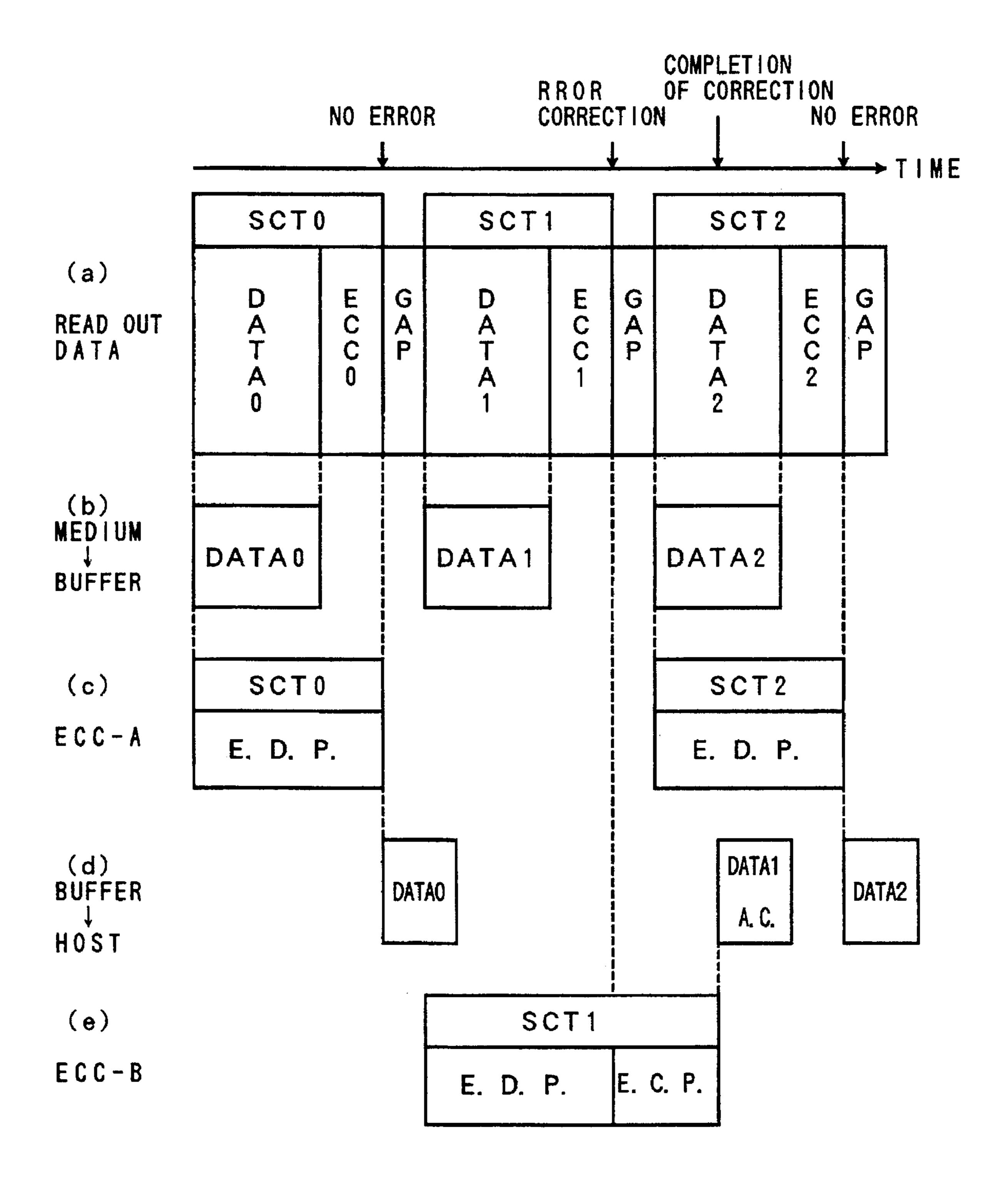
E.D.P.: ERROR DETECTION PROCESSING E.C.P.: ERROR CORRECTION PROCESSING
